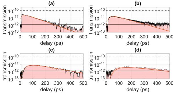
FIG. 4. THG cross-correlation traces obtained for  $[c] = 6.7\%$  (a),  $[c] = 8.3\%$  (b),  $[c] = 13.3\%$  (c) and  $[c] = 20\%$  (d). All red line fits are extracted from (c) providing  $\mu'_s = (79 \pm 7)[c] \text{ cm}^{-1}$  and based on Eq 1 with  $\tau = 25 \text{ fs}$ ,  $\delta\Omega = 5.1\pi 10^{-6} \text{ srd}$ . The horizontal solid and dotted grey lines correspond respectively to our detector noise level and the lowest reported in the literature [2, 34]
