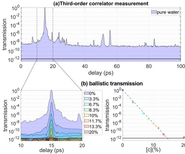
FIG. 3. (a) THG cross-correlation measurement through the cell filled with pure demineralized water and used for reference (b) Same measurement with increasing intralipid-10% concentration  $[c]$  (color coded) zoomed in over a 20 ps time window around the ballistic component centered at  $\sim 15$  ps (left) and linear fit of the peak value using  $\mu_s = (189 \pm 10)[c] \text{ cm}^{-1}$  (right).
