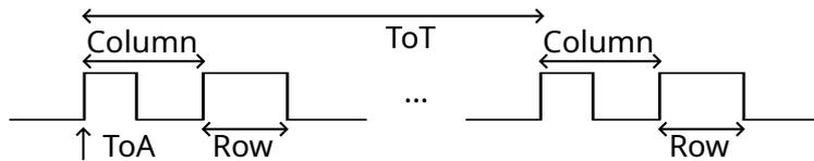
**Figure 2:** Sketch of the delay-based encoding scheme used by the DPTS. Shown is the sequence of pulses originating from a single pixel hit.
