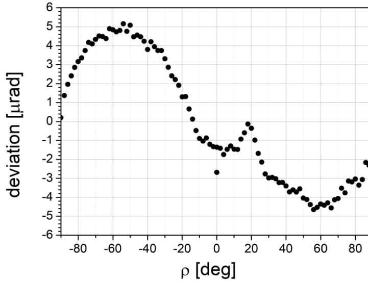
Fig. S1 Experimentally measured deviation of the Ge(111) Bragg angle position versus  $\rho$ -axis rotation. Measurements were performed at an X-ray energy of 22 keV. ID10 DCD operates in the range between 0 and -90 degrees.
