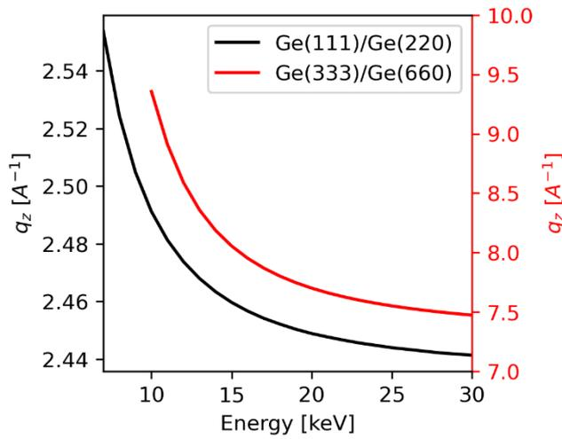
Fig. S2 The value of the  $q_z^{max}$  plotted as a function of X-ray beam energy. The black plot and axis correspond to values calculated for the pair of Ge(111)/Ge(220) reflections. The red plot and axis correspond to values calculated for the pair of Ge(333)/Ge(660) reflections.
