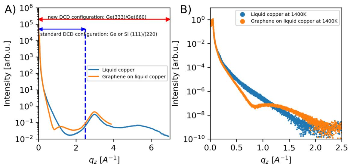
**Figure 6** A) Plot of the scattering intensity as a function of  $q_z$  recorded from bare liquid copper (blue curve) and graphene-covered liquid copper (orange curve) at 1400 K. B) Specular rod, obtained after diffuse background subtraction, of bare liquid copper (red curve) and graphene-covered liquid copper (black curve) at 1400 K.
