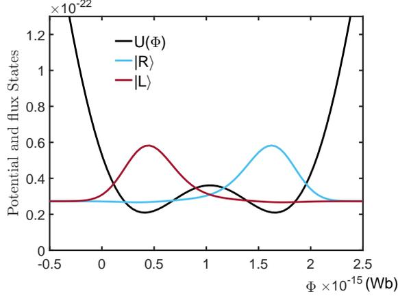
**Figure 12.** The wave functions of the clockwise- (blue line) and anticlockwise (red line) supercurrent states, localized respectively in the left- and right wells of the symmetric potential. The parameters are the same as those used in Fig. 11
