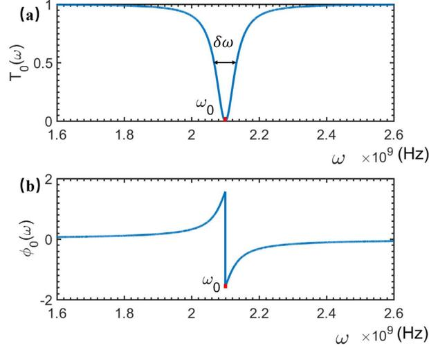
**Figure 2.** The transmitted and phase shift spectra of the travelling microwave scattered simply by the rf-SQUID-based qubit. Here, the relevant parameters are typically set as:  $\omega_0 = 2.1 \times 10^9 \text{Hz}$ ,  $\gamma_c = 3.3 \times 10^7 \text{Hz}$ , and  $\delta\omega = 6.6 \times 10^7 \text{Hz}$ .
