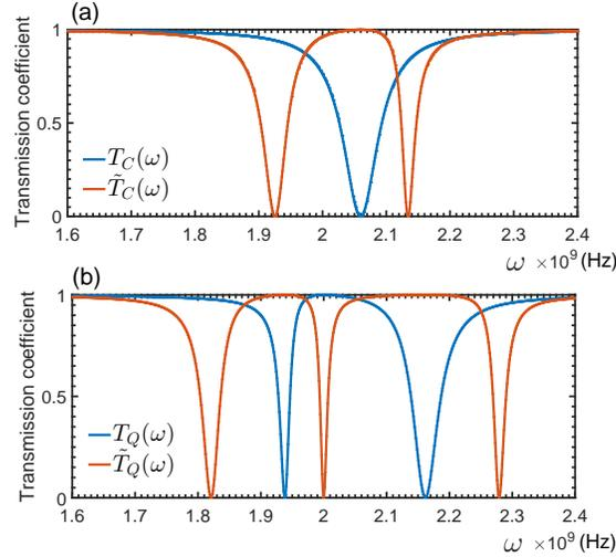
**Figure 10.** Compared the change of transmission peak with or without a resonator, (a)The transmission spectrum contrast of NMR in classical vibration with or without STLR, (b)The transmission spectrum contrast of NMR in quantum vibration with or without STLR,  $\omega_r = \omega_b = 2 \times 10^9 \text{Hz}$ ,  $v_g = 3 \times 10^8 \text{m/s}$ ,  $\omega_0 = 2.1 \times 10^9 \text{Hz}$ ,  $V_2 = 10^8 \text{Hz}$ ,  $g_{rq} = 10^8 \text{Hz}$ ,  $g_C = g_Q = 1 \times 10^8 \text{Hz}$ .
