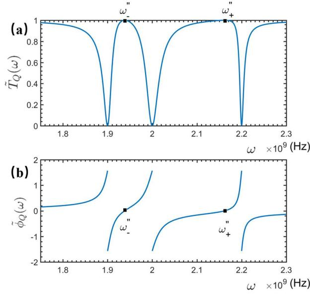
**Figure 8.** The transmitted and phase shift spectra of the travelling microwave scattered by the STLR-qubit-QNMR system. The relevant parameters are set as:  $\omega_r = \omega_b = 2 \times 10^9 \text{Hz}$ ,  $v_g = 3 \times 10^8 \text{m/s}$ ,  $\omega_0 = 2.1 \times 10^9 \text{Hz}$ ,  $V_2 = 10^8 \text{Hz}$ ,  $g_{rq} = 10^8 \text{Hz}$ , and  $g_Q = 1 \times 10^8 \text{Hz}$ .
