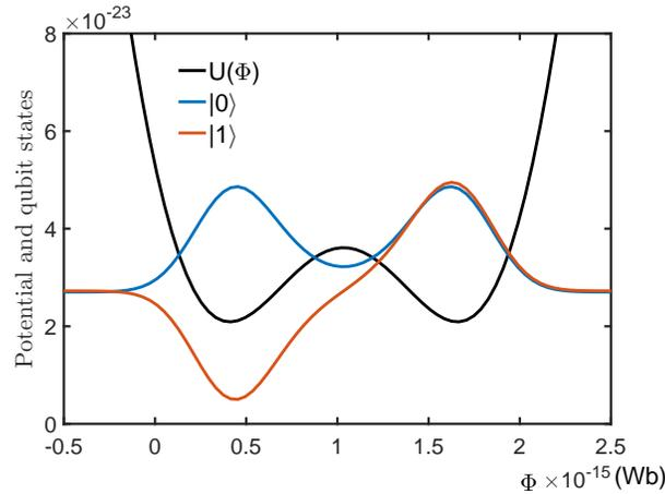
**Figure 11.** Potential function (black line) of a rf-SQUID loop, and the two lowest energy eigenfunctions (blue- and red lines) of the Hamiltonian  $\hat{H}_0$ . Here, the parameters are typically set as:  $\Phi_e = 0.5\Phi_0$ ,  $L = 6 \times 10^{-9}$ H,  $I_c = L\Phi_0/\pi$  and  $C_J = 1.7 \times 10^{-14}$ F, respectively.
