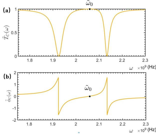
**Figure 9.** The transmitted (a) and phase shift (b) spectra of the travelling microwave scattered by the STLR-qubit-CNMR system. Here, the relevant parameters are set as:  $\omega_r = \omega_b = 2 \times 10^9 \text{Hz}$ ,  $v_g = 3 \times 10^8 \text{m/s}$ ,  $\omega_0 = 2.1 \times 10^9 \text{Hz}$ ,  $V_2 = 10^8 \text{Hz}$ ,  $g_{rq} = 10^8 \text{Hz}$ . The red and yellow lines refer to without and with the CNMR, respectively.
