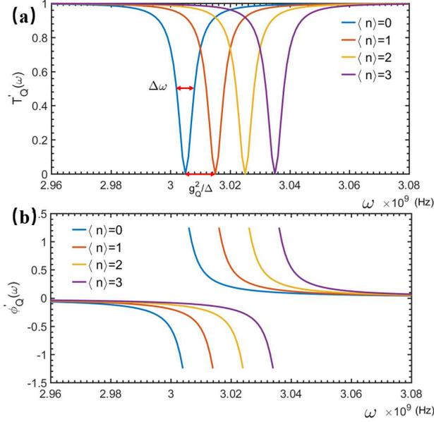
**Figure 4.** (a) Transmitted spectra of probing wave for different average phonon numbers  $\langle n \rangle = 0, 1, 2, 3, \dots$  in the QNMR. (b) Phase shift of probing wave after scattering of qubit dispersively coupled to NMR with different average photon numbers  $\langle n \rangle = 0, 1, 2, 3, \dots$
