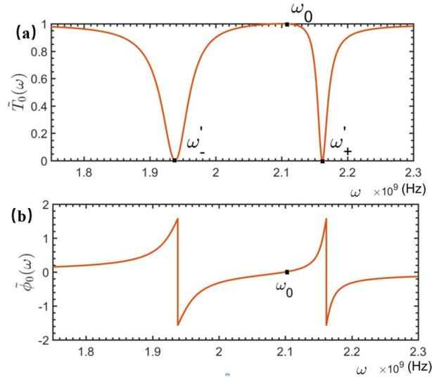
**Figure 7.** The transmitted (a) and phase shift (b) spectra of the travelling microwave scattered by the STLR-qubit system. Here, the relevant parameters are set as:  $\omega_r = \omega_b = 2 \times 10^9 \text{ Hz}$ ,  $v_g = 3 \times 10^8 \text{ m/s}$ ,  $\omega_0 = 2.1 \times 10^9 \text{ Hz}$ ,  $V_2 = 10^8 \text{ Hz}$ ,  $g_{rq} = 10^8 \text{ Hz}$ . The red and yellow lines refer to without and with the CNMR, respectively.
