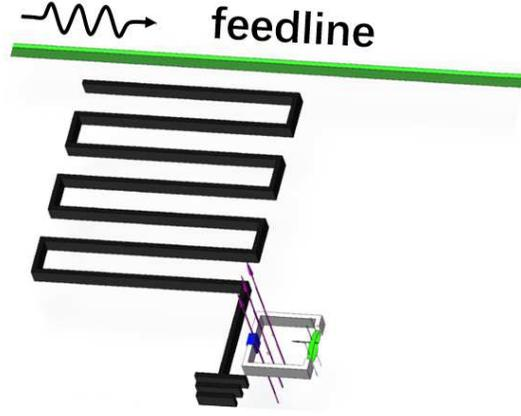
**Figure 6.** Transmitted measurements of the travelling wave scattered by a STLR-qubit-NMR system. Here, the quarter-wavelength STLR is capacitively to the feedline and inductively coupled to the qubit embedded by the NMR.
