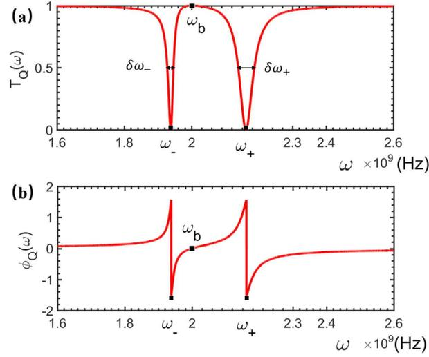
**Figure 3.** The transmitted (a) and phase shift (b) spectra of the travelling microwave scattered by a rf-SQUID-based qubit embedded by a quantum mechanical NMR. The relevant parameters are typically set as:  $\omega_0 = 2.1 \times 10^9$ Hz,  $\omega_b = 2.0 \times 10^9$ Hz,  $\gamma_c = 3.3 \times 10^7$ m/s,  $g_Q = 1 \times 10^8$ Hz.
