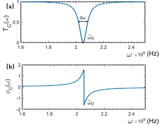
**Figure 5.** The transmitted (a) and phase shift (b) spectra of a rf-SQUID-based qubit embedded by a classical NMR (CNMR). The relevant parameters are set as:  $\omega_0 = 2.1 \times 10^9 \text{ Hz}$ ,  $\omega_b = 2 \times 10^9 \text{ Hz}$ ,  $\gamma_c = 3.3 \times 10^7 \text{ m/s}$  and  $g_C = 1 \times 10^8 \text{ Hz}$ .
