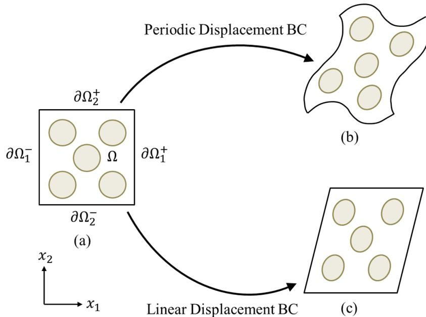
**Figure 2.** Schematic of a 2D RVE and different displacement boundary conditions. (a) The initial configuration of RVE occupying the domain  $\Omega$ , where  $\partial\Omega_{\alpha}^{+}$  and  $\partial\Omega_{\alpha}^{-}$  denote a pair of opposite external boundaries, and  $\alpha = 1, 2$  for this 2D model. (b) The current configuration of RVE subjected to periodic displacement boundary conditions. (c) The current configuration of RVE subjected to linear displacement boundary conditions.
