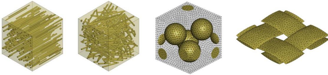
Figure 1. Illustration of the Representative Volume Element (RVE) for composites
