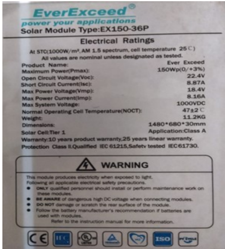
Figure 2: Nameplate of PV panel
