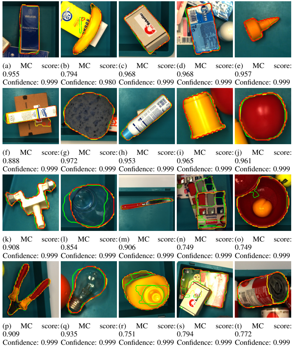
Figure 7: Image examples of objects from the real-world test dataset. The MC score shown is calculated at per object level instead of being averaged over the entire object category. We also show output confidence score for comparison. Gate fusion output is marked in red contour. RGB and depth only are marked in yellow and green contours respectively.
