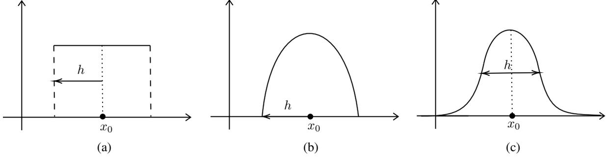
Figure 1: Examples of local kernels: (a) Rectangular kernel  $k(\mathbf{x}) = \mathbb{I}(\|\mathbf{x}\| \leq 1)$ . (b) Epanechnikov kernel  $k(\mathbf{x}) = \frac{d+2}{2V_d}(1 - \|\mathbf{x}\|^2)\mathbb{I}(\|\mathbf{x}\| \leq 1)$ . (c) Gaussian kernel  $k(\mathbf{x}) = \frac{1}{2\pi}e^{-\|\mathbf{x}\|^2}$ .
