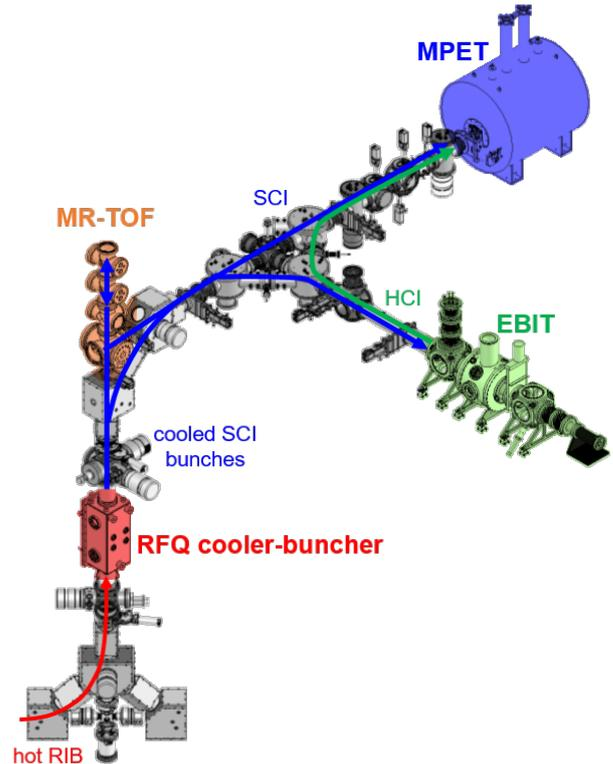
Figure 1: The current TITAN experiment [9] with all traps labelled. Continuous beam is delivered from TRIUMF's Isotope Separator and Accelerator (ISAC) to the RFQ Cooler-Buncher. The beam is then sent to the various other traps for preparation and/or measurement. CID is performed using the MR-TOF-MS.
