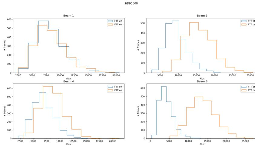
Figure 9: Observation of HD95608 ( $m_V = 4.4$ ): Histogram of the flux injected into the fibers (spectral band 645-900nm). Beams 2 (W2 without Adaptive optics) and 5 (S1 not available at the time of these observations) were closed.
