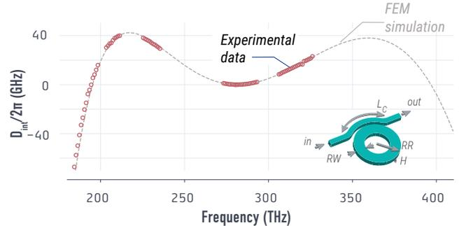
**Fig. S2** Integrated dispersion measurement (red circles) and its comparison against FEM simulations for the ring resonator studied in this work
