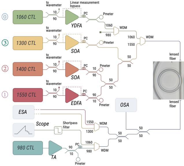
**Fig. S1** Experimental setup used in this work. CTL: continuously tunable laser; YDFA: ytterbium doped fiber amplifier; SOA: semiconductor optical amplifier; EDFA: erbium doped fiber amplifier; TA: tapered amplifier; OSA: optical spectrum analyzer; ESA: electrical spectrum analyzer; PC: polarization controller; Pmeter: power meter; WDM: wavelength division multiplexer
