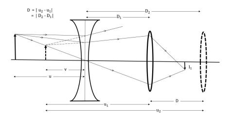
Figure 1: Schematic for a virtual image formation by a concave lens and photographing it by a smartphone camera
