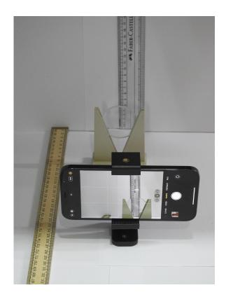
Figure 2: Experimental setup with a concave lens
