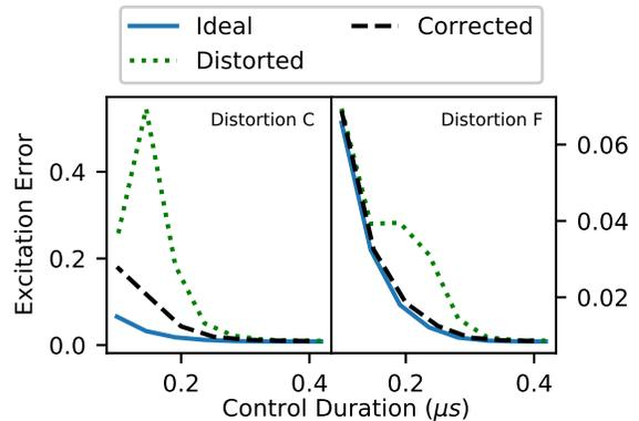
Figure 9. Reduced excitation errors after correcting for the distortion with a gradient-based optimization relying on the trust-region method. (a) distortion C: significant reduced errors, (d) distortion F: mostly recovers the ideal case.
