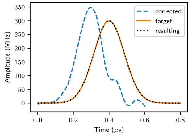
Figure 7. The estimated distortion can be inverted via Eq. (25) and applied to the ideal pulse to produce a pre-distorted pulse. The pre-distorted pulse produces the target Gaussian pulse shape after passing through distortion C.
