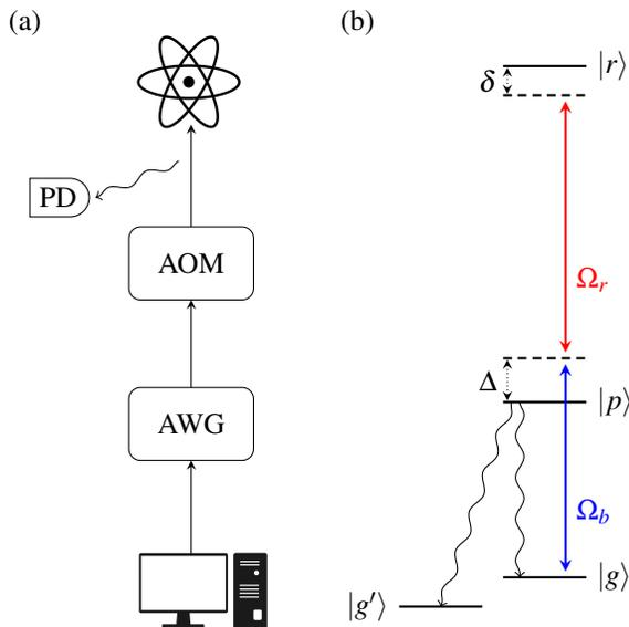
Figure 2. (a) Path of the input control pulse from the computer code via an arbitrary waveform generator (AWG) and an acousto-optic modulator (AOM) to the atom. Before the atom, the output control pulse can be measured using a photodiode (PD). (b) Energy diagram for the excitation of a single Rydberg atom (see text).
