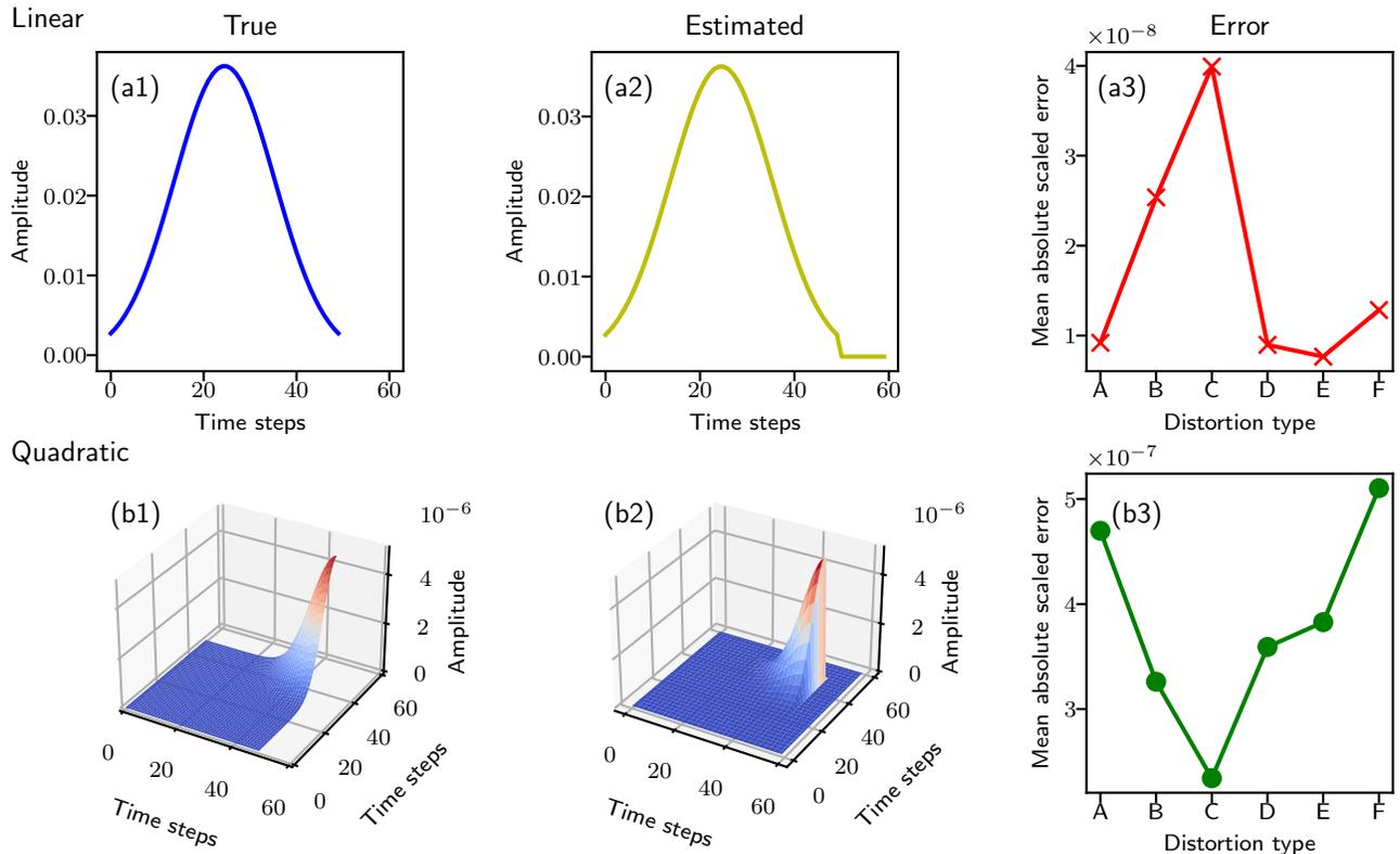
Figure 4. Estimation of both the linear and quadratic components for a non-linear distortion: (a) The linear component (a1) of the distortion C is compared with its estimated value (a2). The amplitude and time steps are dimensionless. (a3) The mean absolute scaled error [as defined in Eq. (22)] between the actual and the estimated values is calculated for various types of distortions A-F [see Eqs. (20)–(21)]. (b) Quadratic component similar as in (a).
