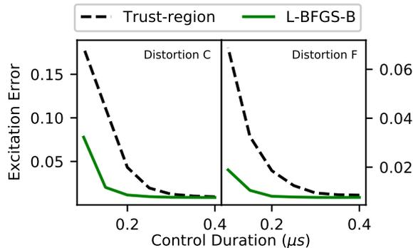
Figure 10. Reduced excitation error for L-BFGS-B when compared to the trust-region method, even though L-BFGS-B does not explicitly enforce constraints on the control pulses (such as limited rise speeds). But the correctly estimated transfer function will implicitly account for pulse constraints. Also, L-BFGS-B is more effective in the optimization.
