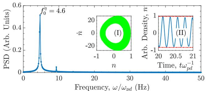
FIG. 2. PSD of the evolution of KdV-B equation with initial perturbation Eq. (4) at  $\eta = 0.0025$ . The time-series of the KdV-B equation is shown in the inset (II). Inset (I) is the phase space plot of the same KdV-B time-series.
