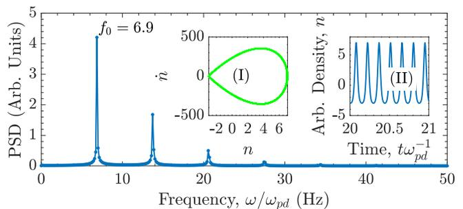
FIG. 1. PSD for the times-series of KdV equation with initial perturbation Eq. (4). Inset (II) shows the time-series obtained from the evolution of the KdV equation. Inset (I) is the phase space plot for the same time-series.
