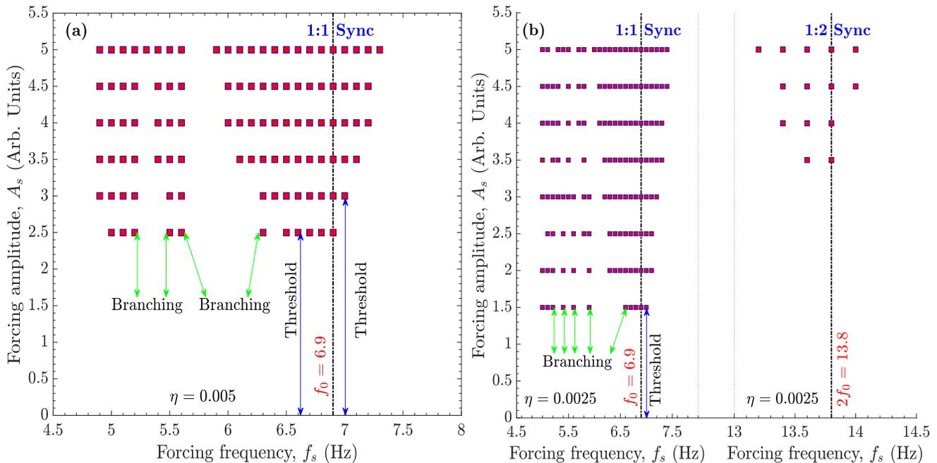
FIG. 5. The Arnold tongue diagrams for (a) harmonic (1:1) synchronization state with  $\eta = 0.005$  and (b) harmonic (1:1) and super-harmonic (1:2) synchronization states with  $\eta = 0.0025$  in the fKdV-B model. In subplot (a) the amplitude is varied from  $A_s = 0.25A_0$  to  $A_s = 0.50A_0$  for 1:1 synchronization. In subplot (b) the amplitude is varied from  $A_s = 0.15A_0$  to  $A_s = 0.50A_0$  for 1:1, and  $A_s = 0.35A_0$  to  $A_s = 0.50A_0$  for 1:2 synchronization.
