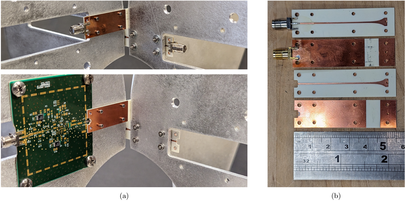
Fig. 4: (a) (Top) Two microstrip baluns terminated by SMA connectors, as installed on each polarization petals of the feed. The balun closest to the backshort is labeled “polarization 0,” and the one closest to the exponential taper is labeled “polarization 1.” Not shown: the short to the petal, on the other end, which is done through an off-the-shelf connection pin. (Bottom) Alternate microstrip baluns without SMA connectors, with a custom CHORD amplifier on one plane. A box covering the amplification circuit was removed for the picture. (b) The two different types of microstrip baluns, before being installed on the feed.
