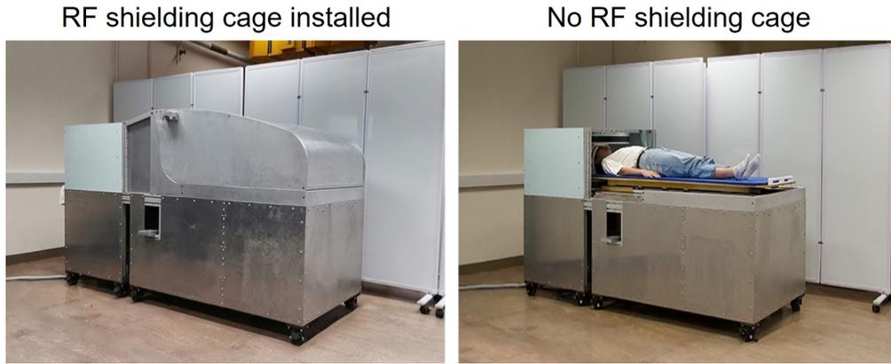
**Figure 2.** Experimental setups for quantitatively assessing the effectiveness of the proposed EMI cancellation method in eliminating EMI related image noise for 0.055 T mobile MRI scanner. For comparison, a custom-made RF shielding cage (consisting of aluminum covers) was installed to fully enclose the subject, or removed.
