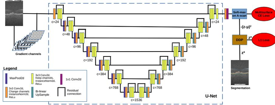
**Fig. 1.** The U-Net based network architecture with additional seven gradient channels as input. The number of channels for each layer is indicated with  $c$ . The DDP module solves the optimization problem for segmentation and outputs optimal smooth retinal surfaces  $\mathcal{S}$  for the  $L_1$  loss.
