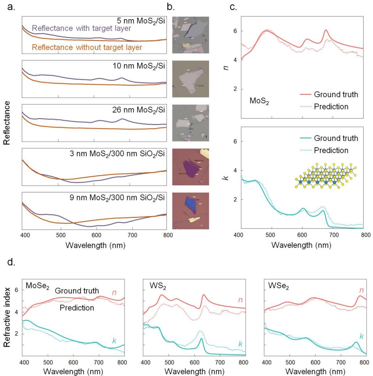
**Figure 3. Predictions of complex refractive indices on experimentally measured reflectance spectra for exfoliated 2D materials.** (a) 5 pairs of reflectance spectra of different multilayer stack structures with and without the exfoliated MoS<sub>2</sub> as the target layer. (b) The corresponding optical microscopic images of MoS<sub>2</sub> with different thicknesses, and on bare silicon (first three rows) and
