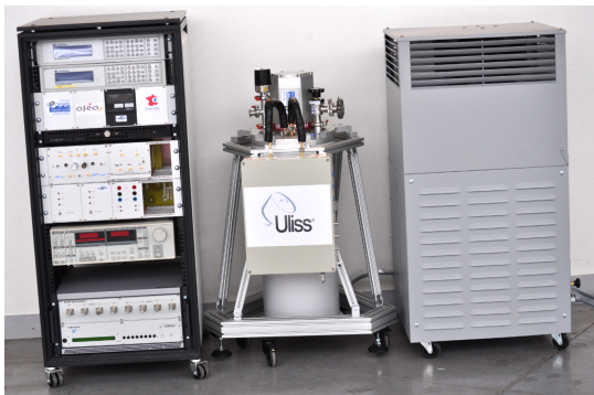
Fig. 10. The CSO of 1 st generation: ULISS-1G. From the left: 19" rack including the electronic and temperature servos as well as the frequency synthesis, the cryostat with the sustaining stage in the front box, and the air cooled He compressor. This unit was designed to be transported in a small van to be tested in different sites around Europe. In Femto-ST, the CSO are running with a water cooled compressor.
