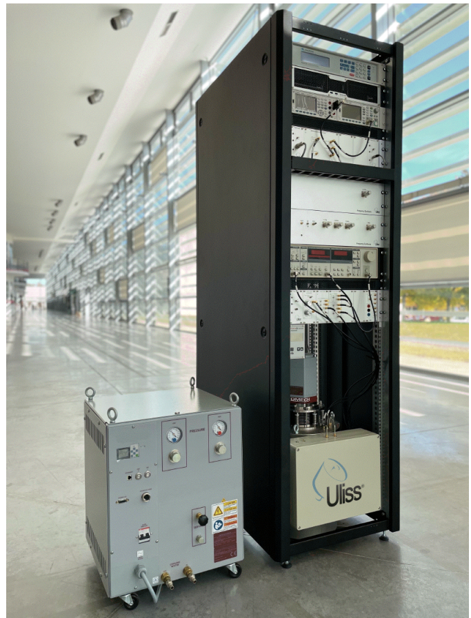
Fig. 11. The CSO of 2 nd generation: ULISS-2G. Its electrical consumption is 3 kW single phase.
