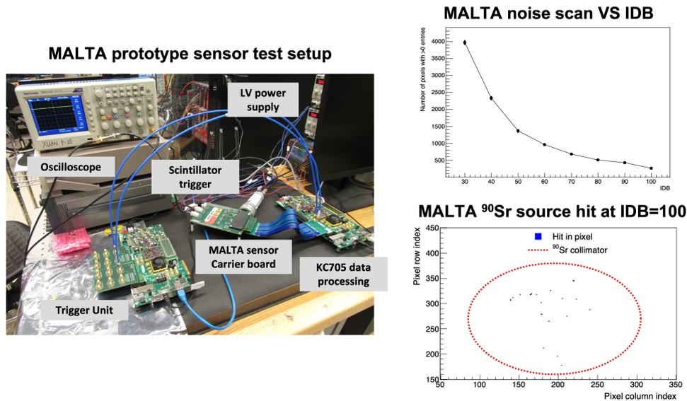
**Figure 5:** The MALTA prototype sensor bench test configuration (left), the MALTA noise scan versus the IDB parameter (top right) and  $^{90}\text{Sr}$  source hit occupancy in a MALTA prototype sensor with the IDB value at 100 (bottom right).
