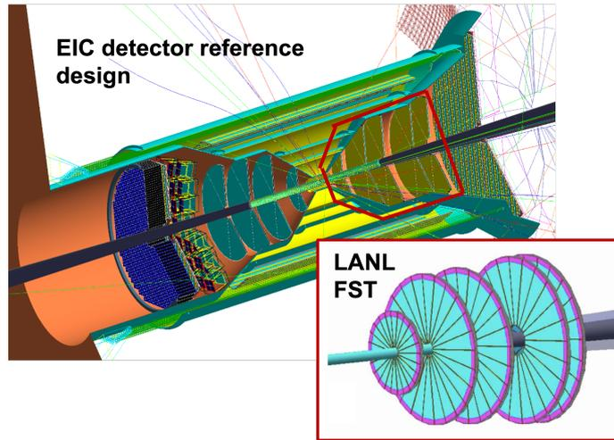
**Figure 1:** The Forward Silicon Tracker (FST) [3, 4] geometry has been implemented in GEANT4 simulation as highlighted inside the red box. The FST design, which consists of detailed layout of the segmented silicon sensor wedges, readout modules and basic support structure, has been included in the EIC detector reference design [5].
