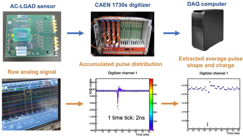
**Figure 3:** The data processing and digitization scheme for AC-LGAD prototype sensor  $^{90}\text{Sr}$  source tests. The readout chain starts with the analog outputs from the AC-LGAD sensor (top left), performs signal digitization with the CAEN 1730s digitizer (top middle) and carries out monitoring and final data processing in the DAQ computer (top right). The analog and digital data outputs for each step is shown in the bottom row.
