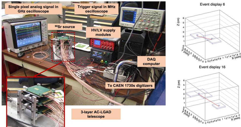
**Figure 4:** The configuration of the 3-layer AC-LGAD telescope  $^{90}\text{Sr}$  source tests is shown in the left and two event displays of tracks reconstructed with this telescope in  $^{90}\text{Sr}$  source tests are shown in the right.
