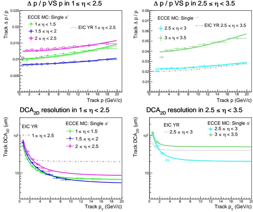
**Figure 2:** The tracking performance of the EIC detector reference design in the pseudorapidity region of  $1.0 \leq \eta \leq 3.5$ . The track momentum dependent momentum resolution (top panel) and the track transverse momentum dependent transverse Distance of Closest Approach ( $DCA_{2D}$ ) resolution in different pseudorapidity bins are compared with the EIC yellow report requirements [1]. These performance results are evaluated with the 1.4 T Babar magnet.
