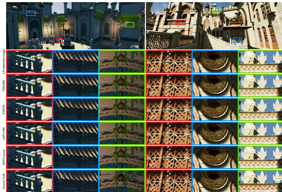
Fig. 7. Qualitative comparison of different methods using representative images from our test datasets. The SR factor is 3. Compared with \times 2 SR, a larger SR factor brings challenges to all the methods. However, the proposed method can still produce sharp edges. This is mainly attributed to its paradigm of predicting offsets.
