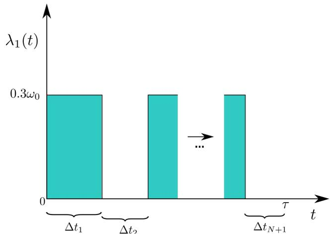
FIG. 3. Example of an optimal control PMP candidate (36) with  $N$  switches for the single-qubit DCP problem with  $\mathbf{x} = (1, 0, 0)$  and  $\lambda_1^{\min} = 0$ : it corresponds to a Bang-Bang function that oscillates between 0 and  $\lambda_1^{\max}$  at the switching times  $t_k$  of the selected partition (35).
