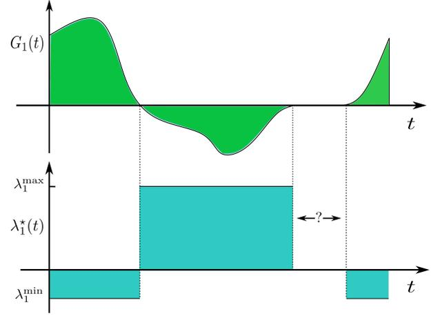
FIG. 2. Example of the relationship between a time-optimal control  $\lambda_1^*(t)$  and the  $G_1(t)$  function for the case in which the system is characterized by a single control function ( $m = 1$ ). The region with a question mark is a singular interval, where the value of the optimal control is not determined by the conditions in Eq. (22).
