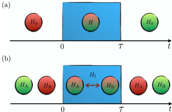
FIG. 1. a) Direct Charging Process: charging model for a closed system through the modulation of an external control for a finite amount of time  $\tau$ . b) Mediated Charging Process: it consists in letting two systems A and B interact through an Hamiltonian  $H_1$ .
