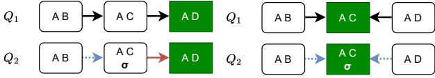
(a) Message passing to root AD. (b) Moving the root increases message reuse.
