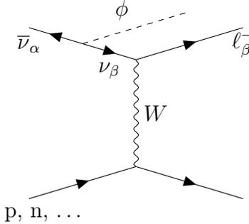
**Figure 5:** Feynman diagram relevant to the mono-neutrino signal. Note that the hadronic current can go beyond nucleon level (e.g. two-body currents, deep inelastic scattering), so we leave it general.
