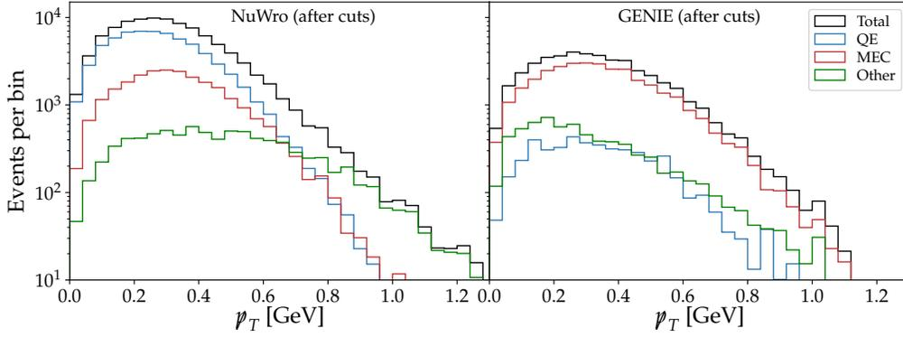
**Figure A3:** Missing transverse momentum spectrum broken down by neutrino-nucleus cross section process for NuWro (left) and GENIE (right), after experimental cuts. The cuts select events with exactly one proton above 100 MeV, no neutrons above 100 MeV and no pions.
