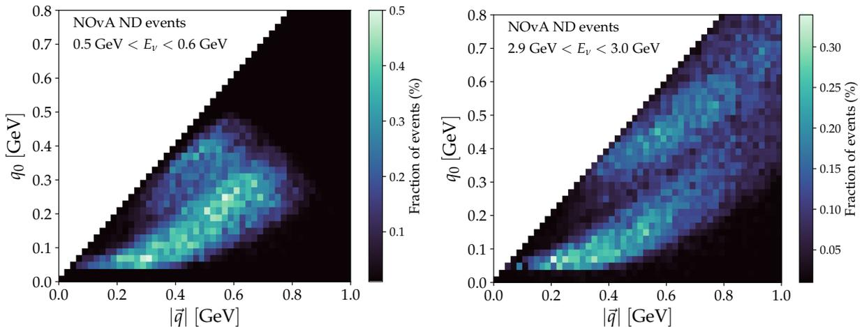
**Figure A2:** Normalized distribution of charged current  $\nu_\mu$ -carbon events at NOvA for  $E_\nu \in [0.5, 0.6]$  GeV (left panel) and  $E_\nu \in [2.9, 3]$  GeV (right panel). The large overlap for these two disparate energies shows the lack of correlation between neutrino energy and NOvA’s tuning variables.
