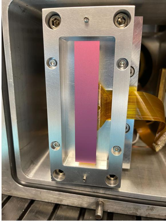
Figure 5: Thick AstroSkipper CCD packaged at Fermilab (detector is inside carrying box). The AstroSkipper CCD and carrying box have been mounted inside of the vacuum chamber for testing.
