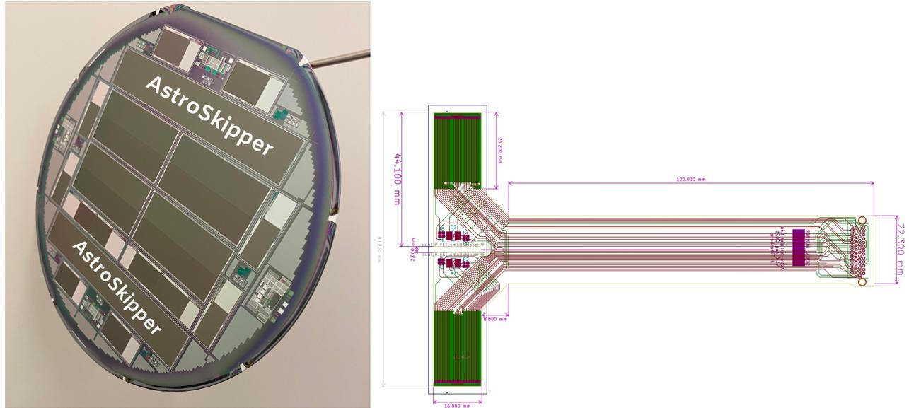
Figure 3: Left: Silicon wafer containing 16 Skipper CCDs for different Fermilab R&D projects. We will be using the  $6k \times 1k$  pixel CCDs with four amplifiers for the Skipper CCD focal plane (labeled “AstroSkipper”). Right: AstroSkipper flex cable with active components, i.e., two JFETs and resistors. The flex cable uses an Omnetics connector (right edge of the cable).
