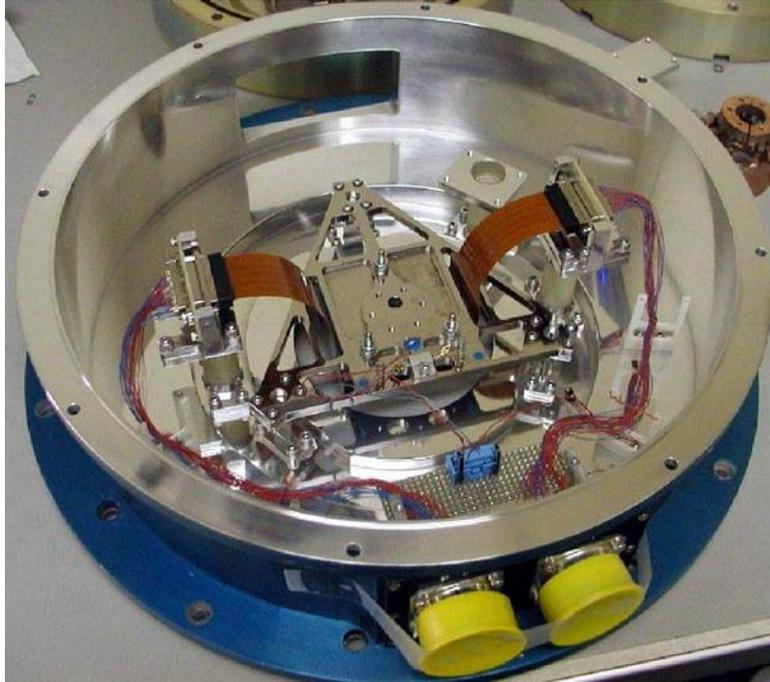
Figure 8: Current SIFS Detector mount, designed for a single e2v CCD44-82 ( 4 K×4 K). The image show the detector, and below it, the mount, which is a triangular aluminum plate that attaches to the dewar through three posts.
