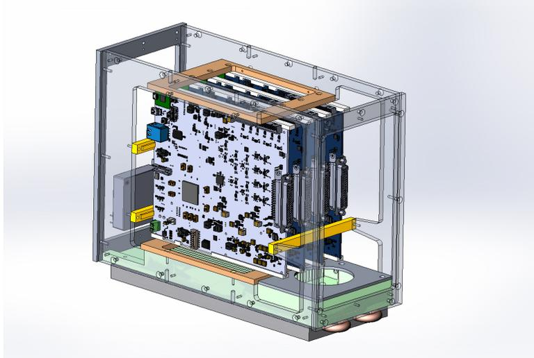
Figure 12: LTA enclosure box for SOAR. It includes a fan for air circulation and a heat exchanger plate, cooled with glycol going through the upper plate (shown at the bottom in the image). The box includes 12V and 5V supplies.
