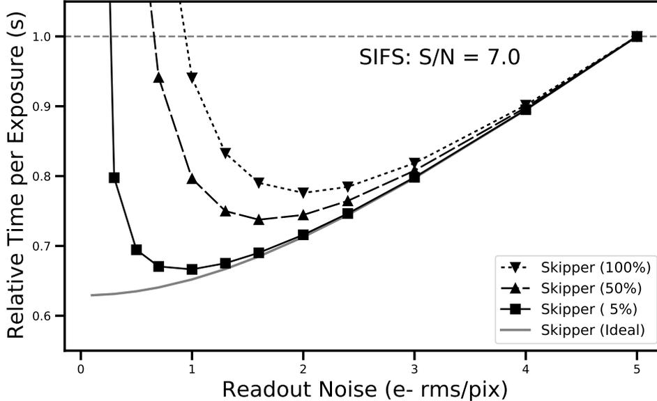
Figure 2: Relative exposure times as a function of detector readout noise at a fixed S/N. Curves represent 100%, 50%, and 5% of the detector being read out.
