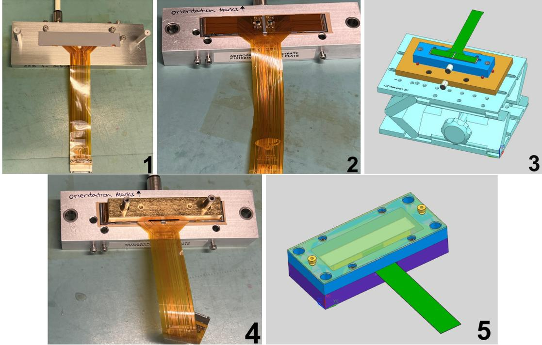
Figure 4: Skipper CCD packaging process. (1) Flex cable, with Omnetics connector at the end, is glued to the Si substrate. (2) The CCD, placed on the blue fixture, is attached to the flex-Si substrate assembly. (3) Wirebonding between CCD pads and flex cable. (4) CCD foot, gold-plated piece, is glued to the CCD. (5) CCD package is installed into a carrying box with removable lid for storage, testing, and transport.
