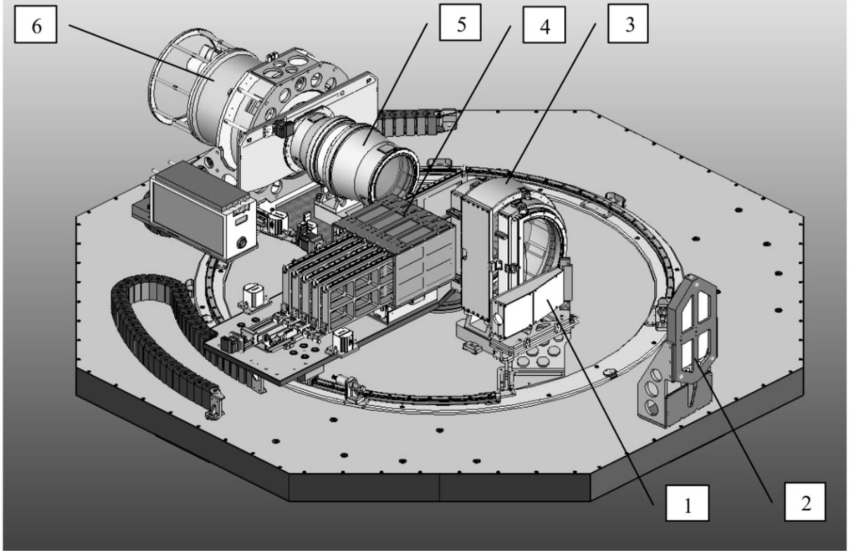
Figure 1: SIFS bench top spectrograph. (1) Output unit support and fold mirror. (2) Collimator mirror. (3) Collimator lenses. (4) VPH grating mechanism. (5) Camera. (6) Cryostat containing detector. (Diagram taken from [13]).
