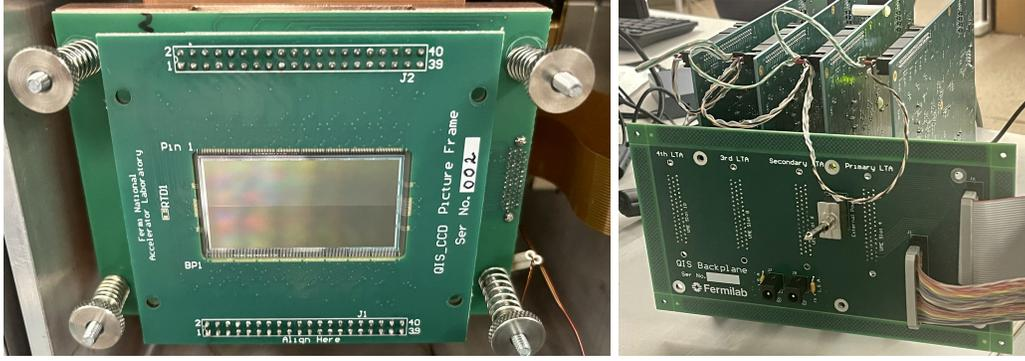
Figure 10: Left:  $2K \times 4K$ , 16 amplifier Skipper CCD. Amplifiers are placed along the long sides of the detector in groups of 8 amplifiers. Right: LTA synchronized readout system used for CCD testing. LTAs are docked to the backplane, which receives the video signals (rainbow ribbon cable) and biases and clocks (grey ribbon cable). Hardware synchronization between boards is done through the cables on the top of the boards.
