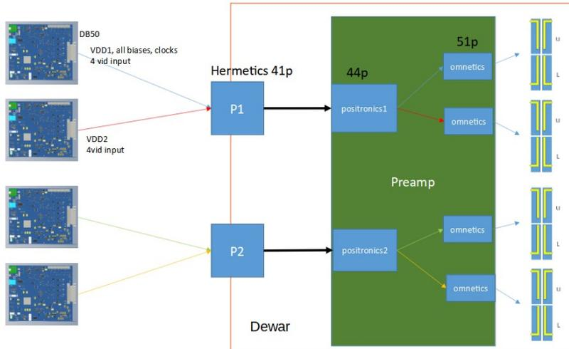
Figure 13: The wiring is designed so that two LTAs handle two AstroSkipper CCDs. This allows for symmetrical cables and independent working, if required for testing purposes. Biases and clocks are shared among two devices, except to VDD.
