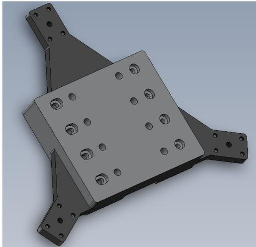
Figure 9: Designed mount for Skippe detectors. It is able to hold 4 AstroSkipper CCDs using the package designed at Fermilab. It uses three ears that allow to use the SIFS head mounting holes.
