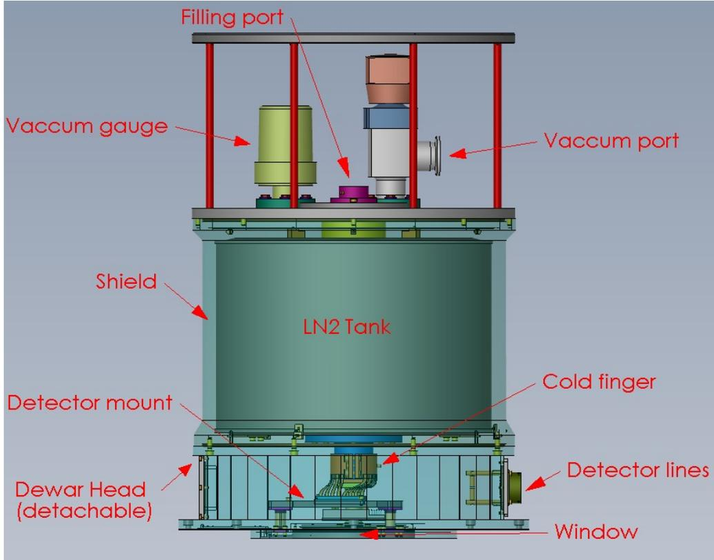
Figure 7: Cross section of a standard SOAR dewar. It uses LN2 to cool the detectors. The detector mount is attached to the tank through a cold finger and a copper piece, with braids trimmed for thermal adjustment.
