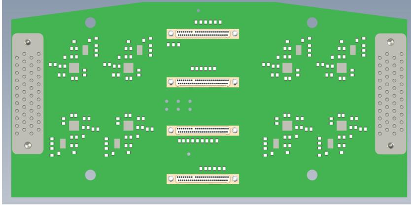
Figure 11: Top side CAD model of the preamplifier PCB board designed at CTIO showing eight of sixteen preamplifiers. The input connectors from the AstroSkipper CCDs are at the center and the output connectors are at the edges.
