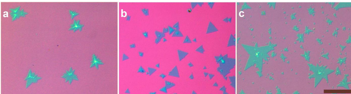
Fig. S-1 Poor (a), moderate (b) and high (c) sample coverage due to the influence of synthesis parameters on the lateral growth. Scale bar is 100 \mu\text{m} .
