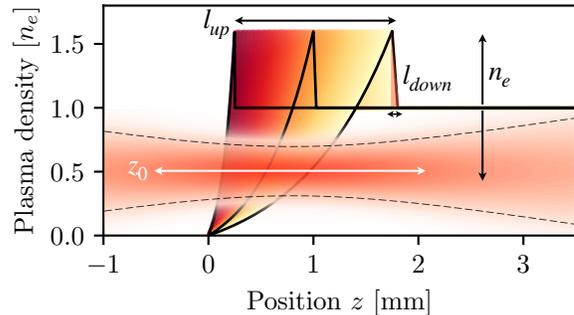
FIG. 1. **Illustration of the four variable input parameters** from Table I, namely the upramp length  $l_{up}$ , the downramp length  $l_{down}$ , the plateau density  $n_e$  and the focus position  $z_0$ .
