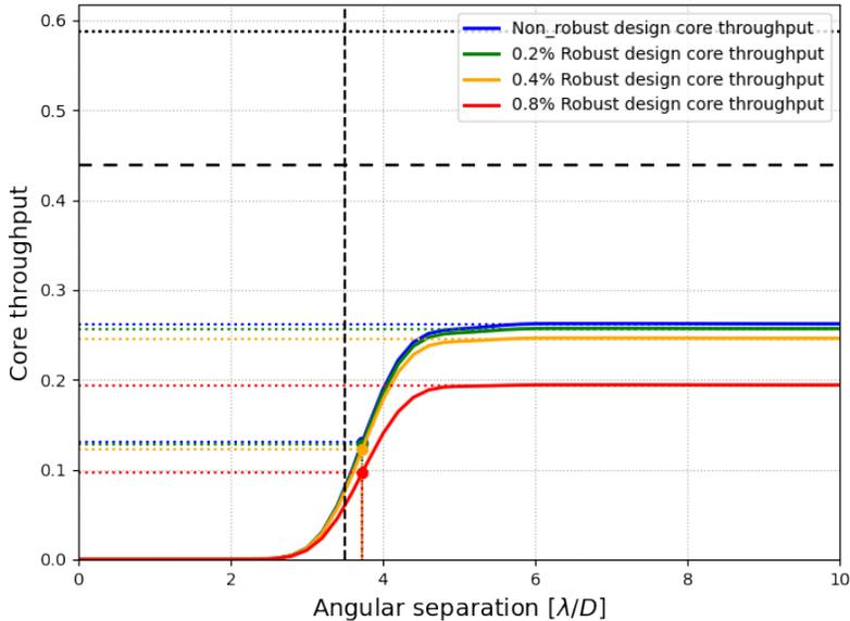
Figure 12. Core throughputs for four 5-Hex designs, one without Lyot stop robustness and three with  $\pm 0.2\%$ ,  $\pm 0.4\%$  and  $\pm 0.8\%$  Lyot stop alignment tolerances, respectively. The plots illustrate the trade-off between design robustness and throughput - increased design robustness results in a corresponding decrease in throughput. Indeed, there is a throughput reduction of 26% between the non-robust design and the design optimized to a LS misalignment tolerance of 0.8%.
