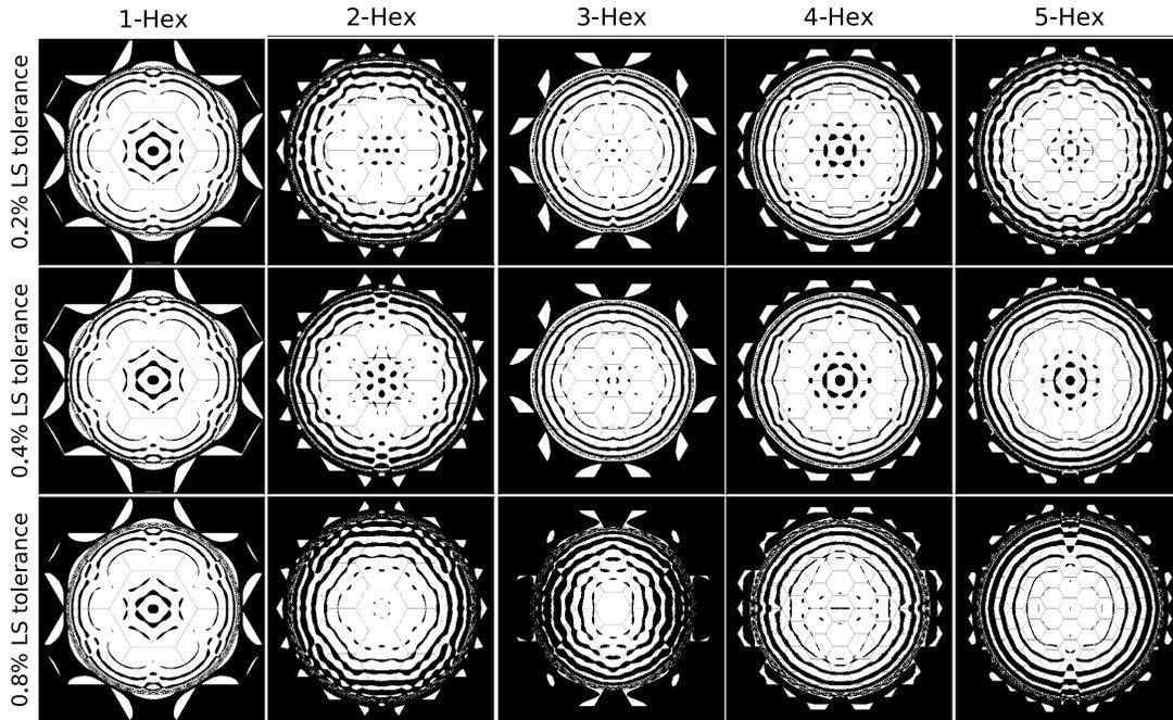
Figure 9. APLC apodizers produced by the N-Hex survey for Lyot stop misalignment tolerances of  $\pm 0.2\%$  (*top*),  $\pm 0.4\%$  (*middle*) and  $\pm 0.8\%$  (*bottom*). These designs produce annular,  $10^{-10}$  contrast dark zones with working angle range 3.4 - 12  $\lambda_0/D$  over a 10% bandpass. *From left:* 1-Hex, 2-Hex, 3-Hex, 4-Hex, and 5-Hex.
