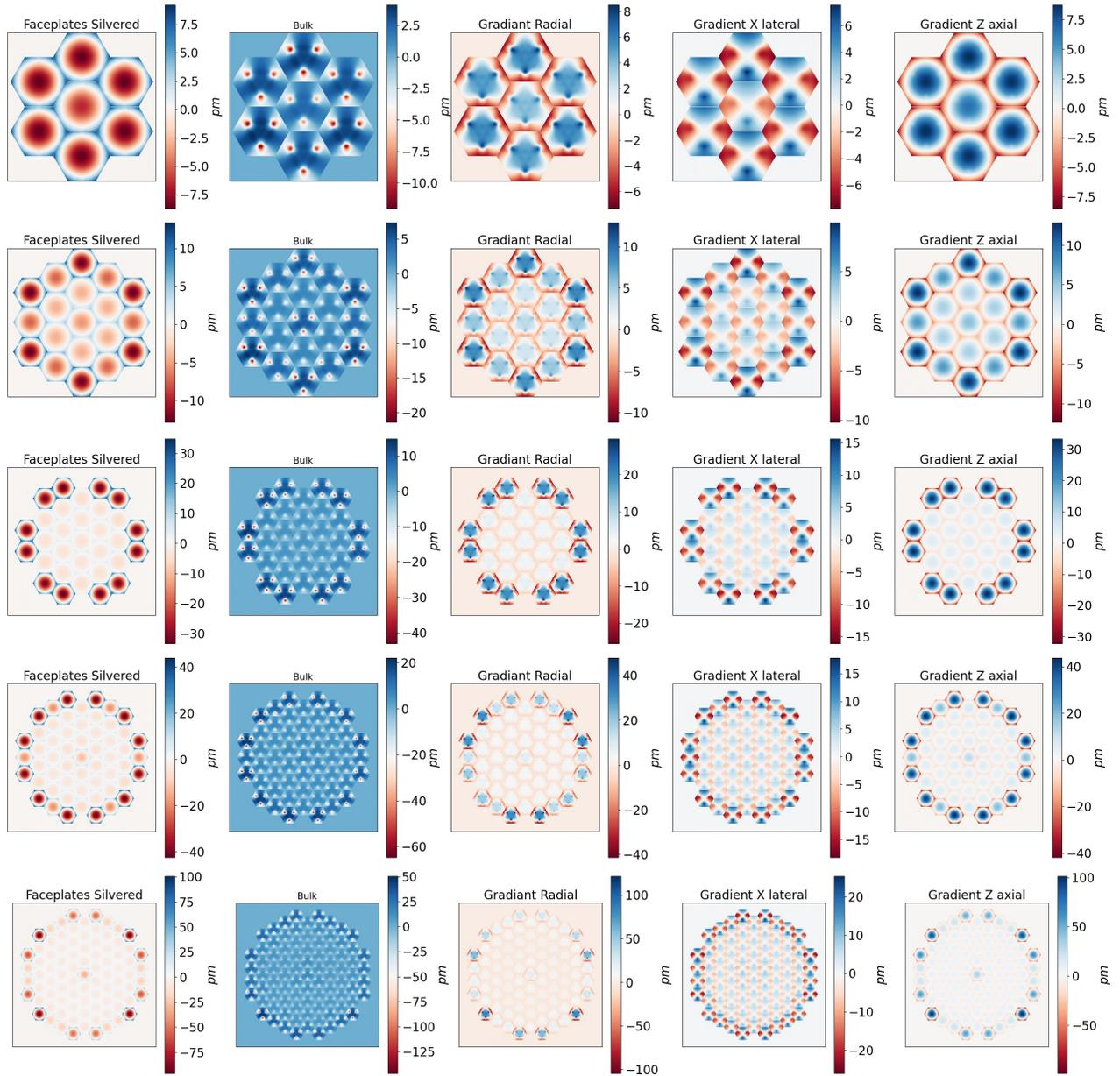
Figure 15. Static surface tolerances caused by temperature changes on the individual segments for five different hexagonal aperture geometries and APLC designs. These results are based on the PASTIS sensitivity analysis of all five thermal modes combined (faceplate, bulk, and thermal gradients),<sup>21</sup> and we obtain the temperature tolerance for each segment to reach  $10^{-10}$  contrast in the dark hole.
