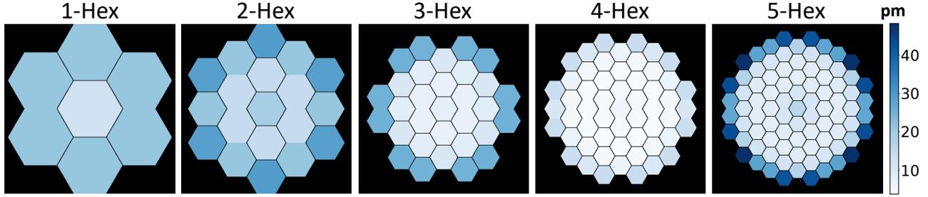
Figure 13. Static piston tolerance for each design from 1-hex to 5-hex, which derives from the PASTIS sensitivity analysis.<sup>18-20</sup> The values for each of these segment correspond to the standard deviation of the surface piston error for each segment with a target contrast of  $10^{-10}$ . All five tolerance maps are plotted on the same scale.
