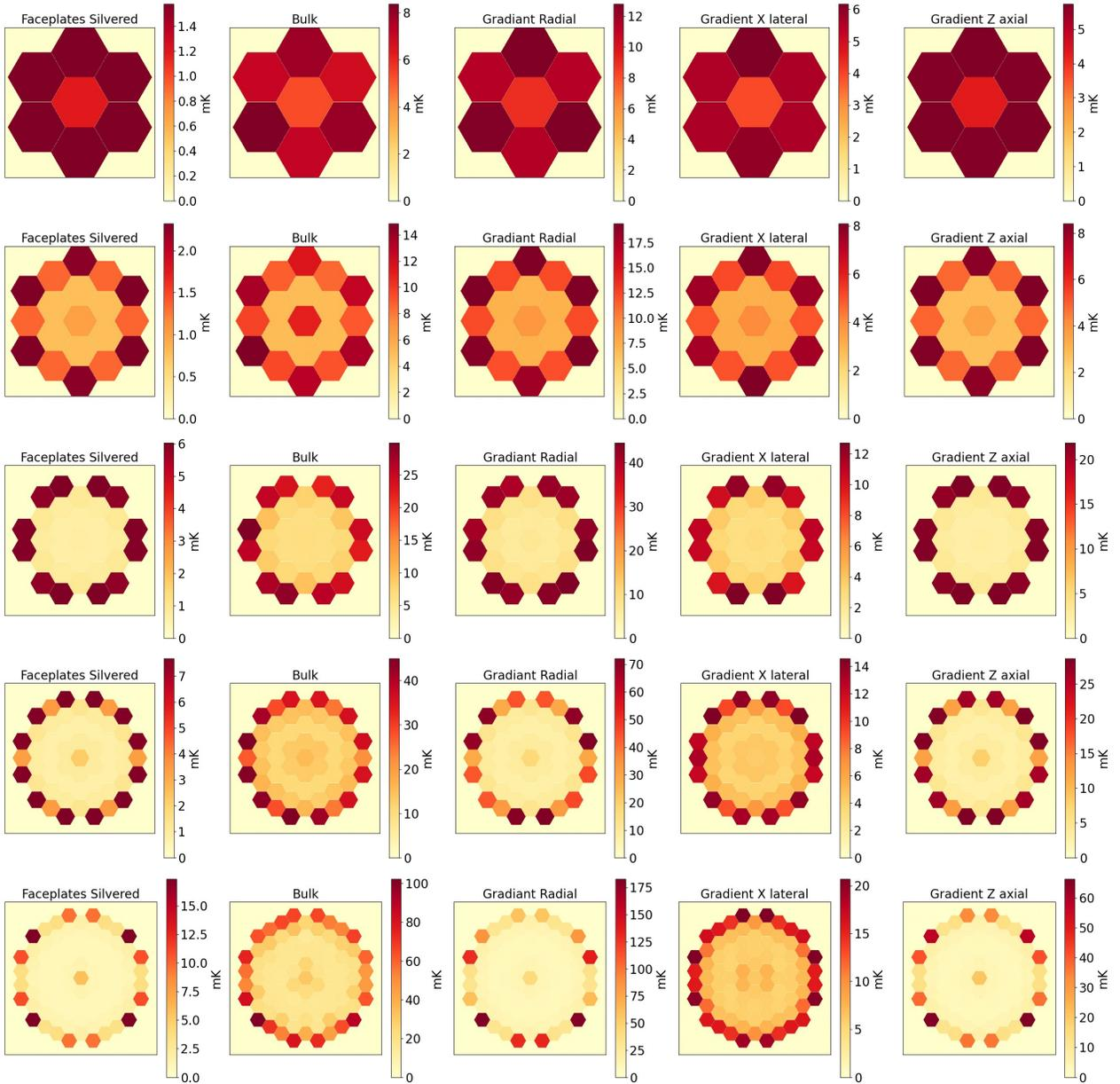
Figure 16. Static, per-segment temperature gradient tolerances for five different hexagonal aperture geometries and APLC designs. These results are based on the PASTIS mode analysis of all five thermal modes combined (faceplate, bulk, and thermal gradients) for currently envisioned hexagonal segments,<sup>21</sup> and we obtain the temperature tolerance for each segment to reach  $10^{-10}$  contrast in the dark hole.
