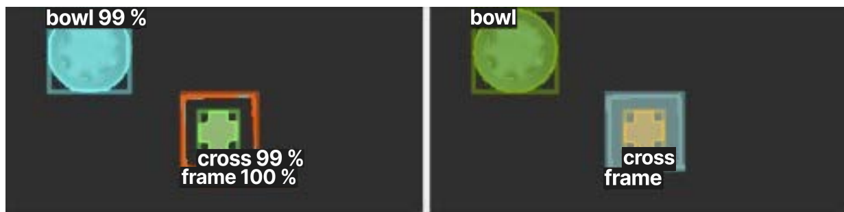
Figure A.20: Visualization of fine-tuned mask R-CNN. Left : Prediction from the detection model. Right : Ground-truth scene parsing. The detection model agrees well with ground-truth objects.
