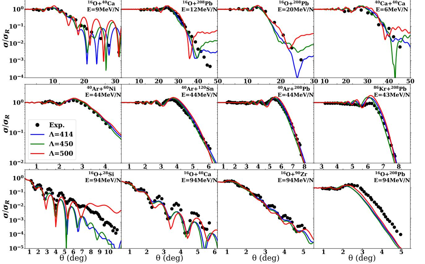
FIG. 2. Elastic scattering cross sections for a selection of medium- and heavy-mass nucleus-nucleus systems at varied energies. Results from  $N^3\text{LO}$  chiral interactions with momentum space cutoffs of  $\Lambda = 414, 450, 500$  MeV are shown in blue, green, and red. Experimental data from Refs. [30–35] are shown as black dots.
