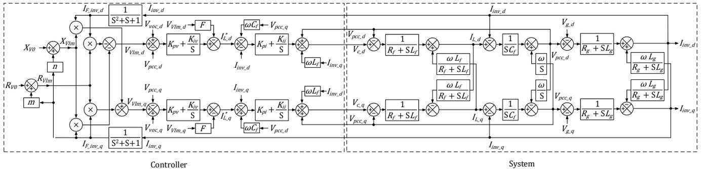
Fig. 4. Small signal model of the system and the controller
