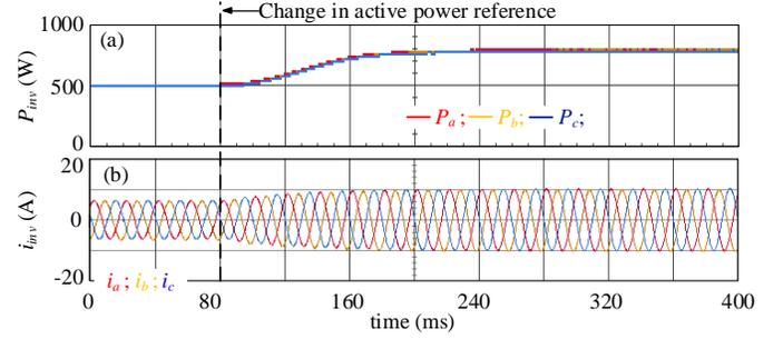
Fig. 12. Normal dispatchable operation of the grid-forming inverter: (a) active power outputs of the individual phases (b) phase currents of the inverter
