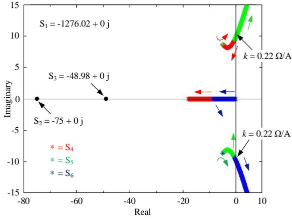
Fig. 5. Eigenvalue loci for the impedance gain,  $k$
