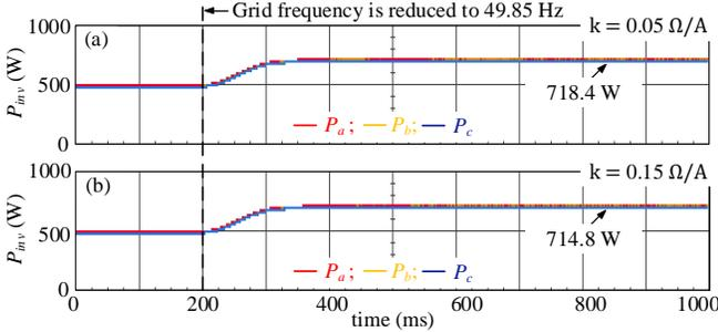
Fig. 15. Active power support by the inverter when the grid frequency reduces to 49.85 Hz from 50 Hz: (a) virtual impedance gain,  $k = 0.05 \Omega/\text{A}$ , (b) virtual impedance gain,  $k = 0.15 \Omega/\text{A}$
