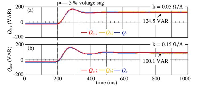
Fig. 13. Reactive power support by the inverter during 5% voltage sag: (a) virtual impedance gain,  $k = 0.05 \Omega/A$ , (b) virtual impedance gain,  $k = 0.15 \Omega/A$
