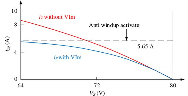
Fig. 7. Quadrature axis current output of the inverter without and with the virtual impedance gain
