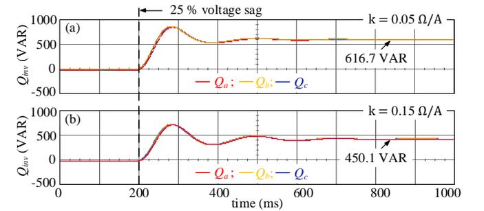
Fig. 14. Reactive power support by the inverter during 25% voltage sag: (a) virtual impedance gain,  $k = 0.05 \Omega/A$ , (b) virtual impedance gain,  $k = 0.15 \Omega/A$
