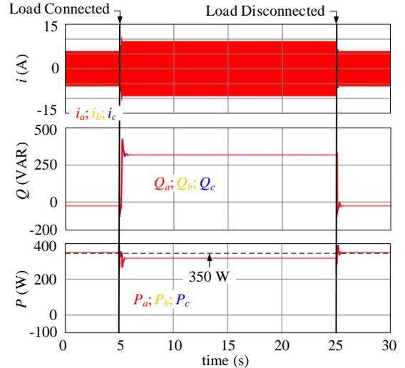
Fig. 8. Performance of a VO-based grid forming controller in the presence of large voltage sag with the proposed voltage stiffness controller
