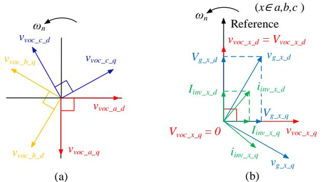
Fig. 3. (a) Output voltage vectors of the S-VOC (b) Instantaneous to synchronous reference frame transformation
