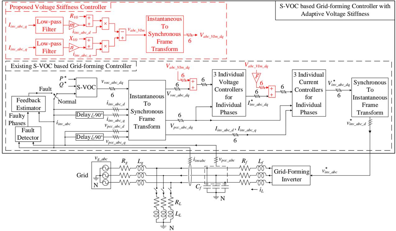
Fig. 1. The schematic diagram of the proposed S-VOC based grid forming controller
