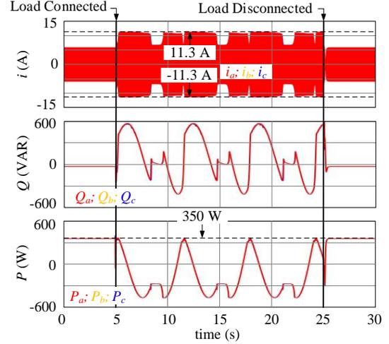
Fig. 6. Performance of a VO-based grid forming controller in the presence of large voltage sag without the proposed voltage stiffness controller
