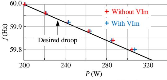
Fig. 9. Active power droop response of the VOC without and with the proposed voltage stiffness controller
