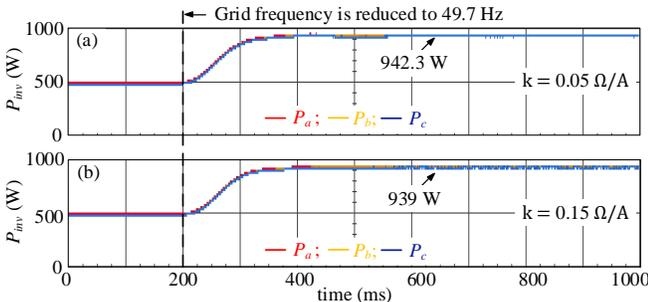
Fig. 16. Active power support by the inverter when the grid frequency reduces to 49.7 Hz from 50 Hz: (a) virtual impedance gain,  $k = 0.05 \Omega/\text{A}$ , (b) virtual impedance gain,  $k = 0.15 \Omega/\text{A}$
