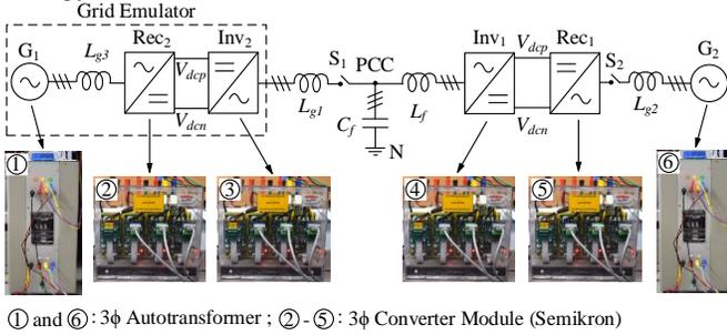
Fig. 10. The schematic diagram of the experimental setup
