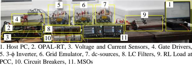
Fig. 11. The picture of the experimental setup
