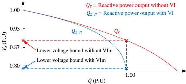
Fig. 2. The reactive power droop characteristic without and with virtual impedance
