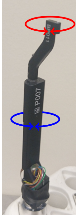
Figure 4: The rotational movements of the arms of a typical astrobot. The red rotation reflects the variable parity of the astrobots since it can rotate in both directions (reprinted with permission[4])
