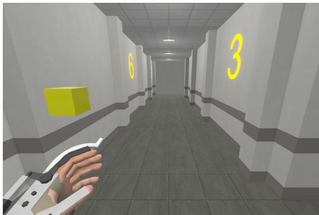
Fig. 2: Screenshot from the virtual environment. The patient is asked to reach the yellow square (target) with the left hand (effector) using motor imagery.
