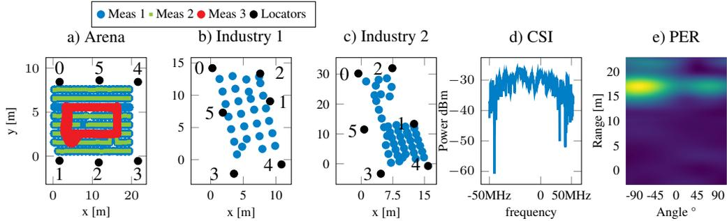
Figure 1: Measurement environments. a) Arena has three different measurement iterations, b) Typical Industrial environment, and c) Harsher industrial environment with rich scatterers. Data examples: d) CSI and e) PER.
