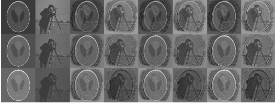
Figure 4.8: Reconstruction of the object for blind polychromatic ptychography with different iteration number setups. Each row corresponds to the single wavelength \ell = 1, 2, 3 . The two consecutive columns are the real and imaginary parts of the mask. In figure, we show the true object z and reconstruction with Algorithm 2 for three choices of (T, l_z, l_w) = (200, 10, 10), (400, 5, 5) and (2000, 1, 1) .
