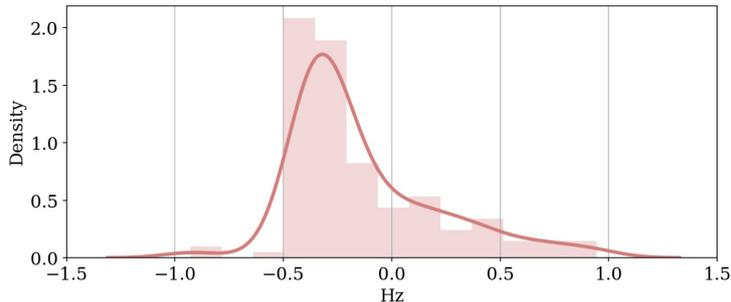
Figure 8: Histogram of the difference between the frequency nadir from the SFR model and the frequency nadir approximation by separable programming for a sample week.
