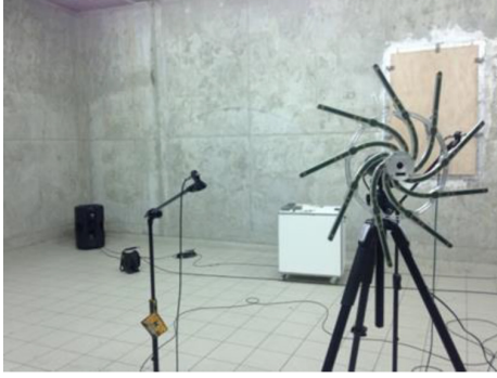
FIG. 4. (color online) Experimental setup: a 43-microphone array in a reverberant room.
