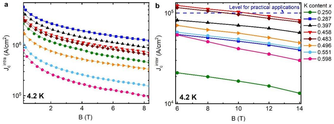
**Fig.2 Critical current density of the  $\text{Ba}_{1-x}\text{K}_x\text{Fe}_2\text{As}_2$  tapes.** Field dependence of the (a) intra- and (b) inter-grain critical current density. The highest  $J_c^{\text{inter}}$  of the measured samples is shown here. The blue dashed line in (b) marks the  $J_c$  level for practical applications. The legend is shown in (b).
