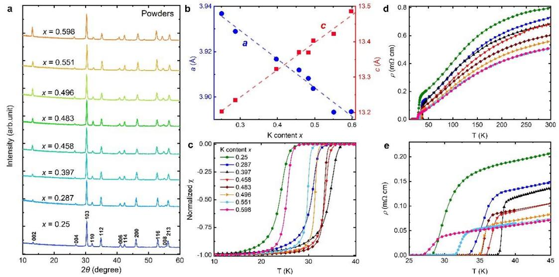
**Fig.1 Crystal structure, susceptibility and resistivity of the  $\text{Ba}_{1-x}\text{K}_x\text{Fe}_2\text{As}_2$  samples.** (a), Powders X-ray diffraction patterns. (b), Doping dependence of the lattice parameters derived from the Rietveld refinements. Temperature dependence of (c) the normalized susceptibility and (d) the resistivity. (e), enlarged view of the resistivity near the superconducting transition. The legend for (c-e) is shown in (c).
