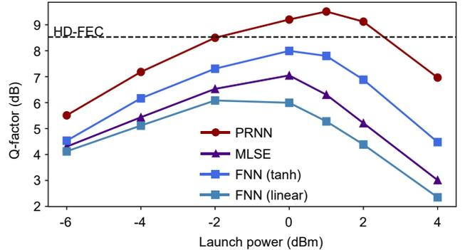
Fig. 3. Comparison of PRNN and various DSP methods in 2-channel 56 GBaud/λ WDM PAM4 signals over 20 km transmission link. PRNN: photonic recurrent neural network; FNN: feed-forward neural network; MLSE: maximum likelihood sequence estimation. tanh: hyperbolic tangent activation function.
