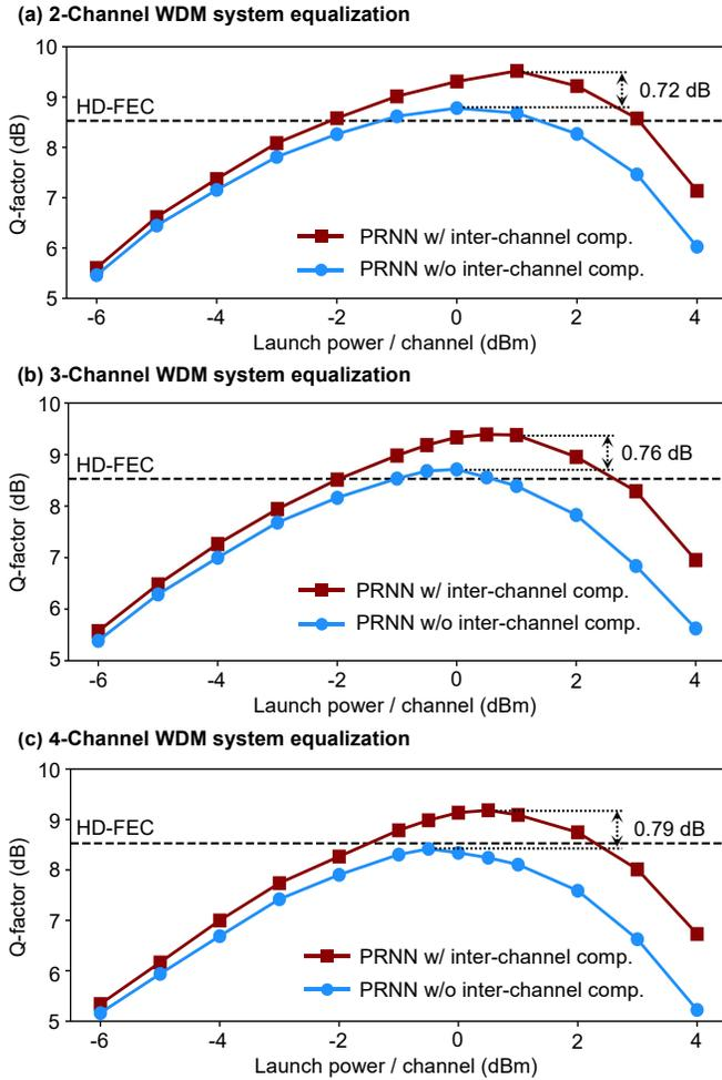
Fig. 4. Equalization performance for (a) 2, (b) 3, and (c) 4 channels WDM systems respectively. The WDM systems have 56 GBaud/ $\lambda$  PAM4 signals up to 20 km transmission with different launch power per channel. The red and blue curves represent the average equalization performance of all channels using PRNN with and without inter-channel nonlinearity compensation, respectively. PRNN: photonic recurrent neural network.
