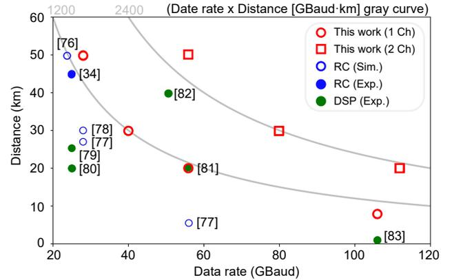
Fig. 5. Comparison of different PAM4 equalization systems with reservoir computing (RC) [34], [76]–[78] and DSP [79]–[83] in terms of data rate and distance. Ch: channel; Sim: simulation; Exp: experiment.
