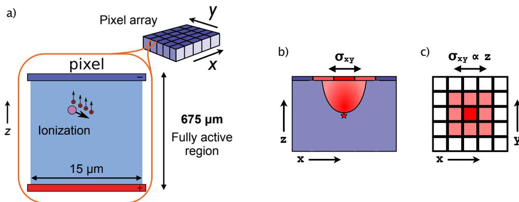
Figure 1: **a)** Sketch of a low-energy particle ionizing the CCD active region. **b)** Diffusion of charge as it drifts toward the pixel array. **c)** The spread of the cluster of charge on the pixel array is positively correlated with the depth of the interaction.
