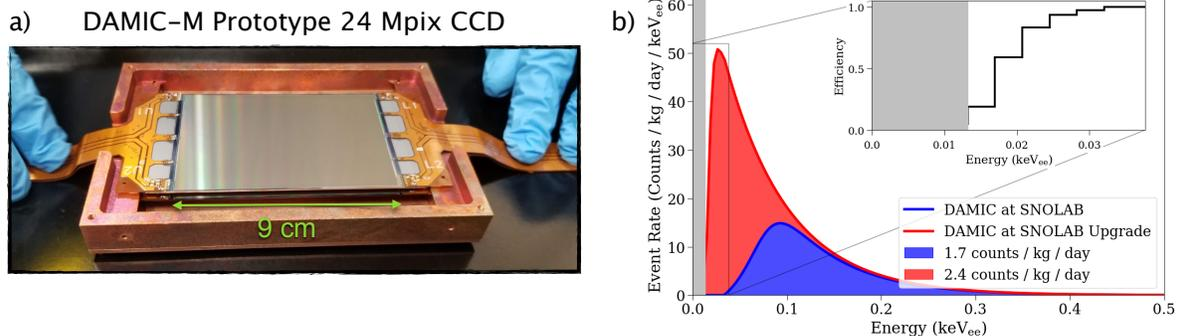
Figure 3: **a)** DAMIC-M 24 Mpix CCDs in their copper storage box. The bottom CCD is barely visible under the top CCD. **b)** Exponentially decaying spectrum of the excess of events observed in DAMIC at SNOLAB. The blue spectrum is the best-fit from the published analysis [3, 13], while the red spectrum is the expectation for the upgraded detector with skipper CCDs. The measured detection efficiency of the upgraded detector (inset) was used to construct the red spectrum.
