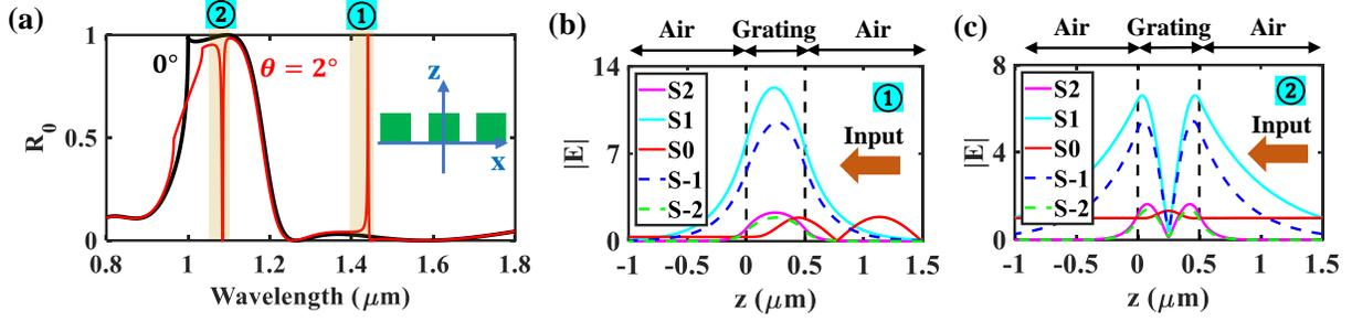
**Fig. 4.** Resonance spectra and leaky-mode profiles under a-GMR. (a)  $R_0$  spectra at  $\theta=0^\circ$  and  $\theta=2^\circ$  of the model 1D optical lattice  $\{\Lambda=1 \mu\text{m}, F=0.5, H=0.5 \mu\text{m}, n=2\}$  at a crosscut of Figs. 4(d) and 4(e) at  $\Lambda=1 \mu\text{m}$ . For a-GMR reflectance peak and null at ① and ②, the corresponding leaky-mode profiles are presented in (b) and (c).
