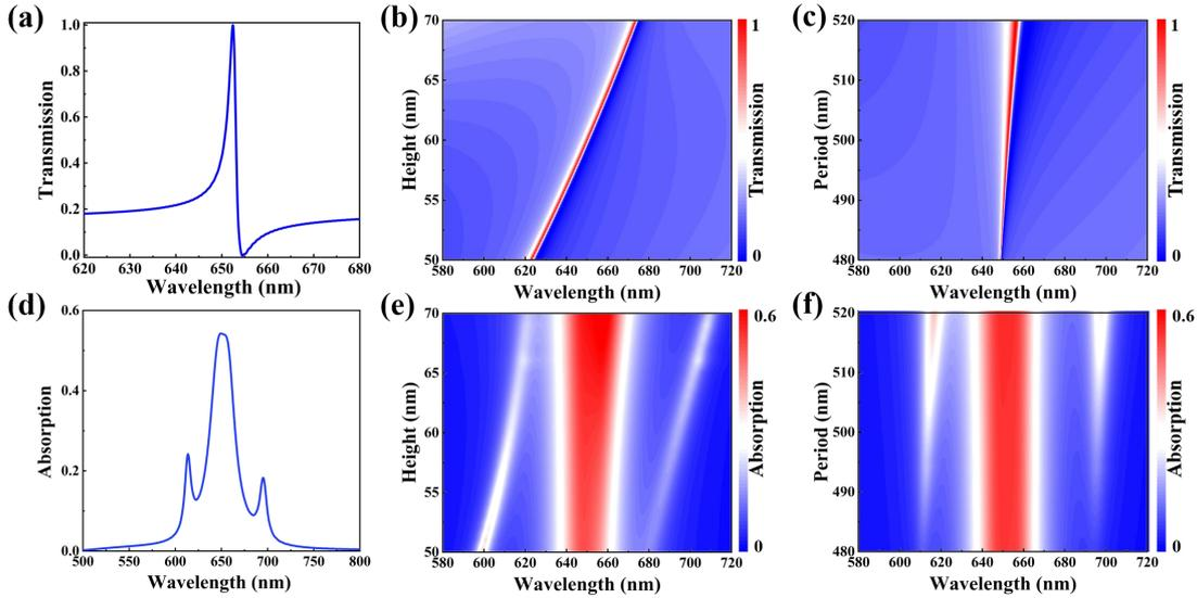
FIG. 3. (a) The transmission spectrum of the quasi-BIC with  $g = 127$  nm. Transmission spectra of the quasi-BIC with respect to (b) height and (c) period. (d) Absorption spectrum of hybrid mode with gap  $g = 127$  nm and height  $h = 61$  nm. Absorption spectra of hybrid modes at different (e) height and (f) period.
