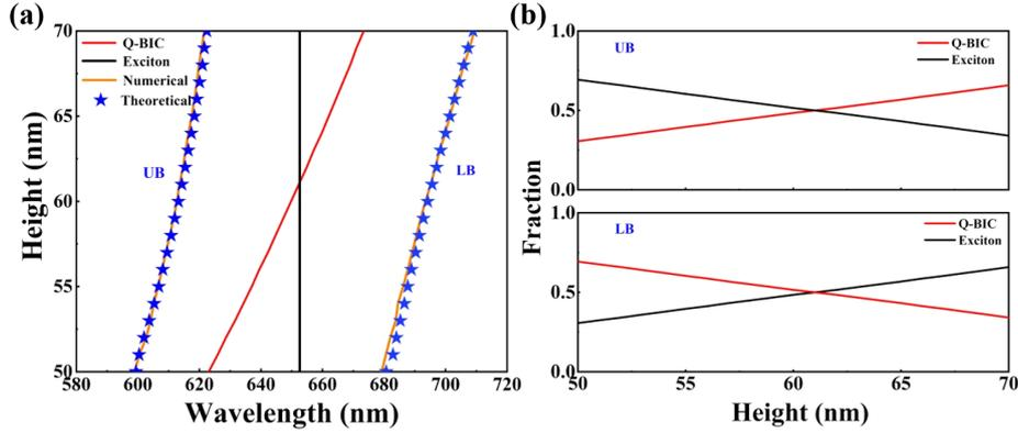
FIG. 4. (a) Theoretical and numerical results of upper branch (UB) and lower branch (LB) of the strong coupling. (b) The fraction curves of exciton (black solid line) and quasi-BIC (red solid line), respectively.
