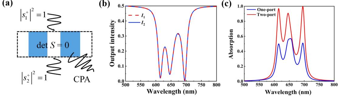
FIG. 6. (a) Schematic diagram of coherent perfect absorption. (b) The output intensities  $I_1$  and  $I_2$  of the system under two-port source excitation. (c) The absorption spectra of the system under one-port and two-port source excitation, respectively.
