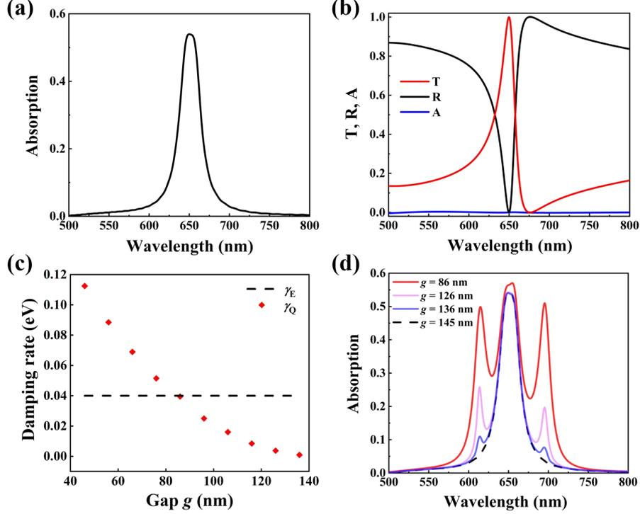
FIG. 5. (a) Absorption spectrum of the grating with  $g = 145$  nm. (b) The transmission, reflection and absorption spectra of the quasi-BIC under  $g = 86$  nm. (c) The damping rate  $\gamma_Q$  and  $\gamma_E$  as the functions of  $g$ . (d) The absorption spectra of the gratings with different  $g$ .
