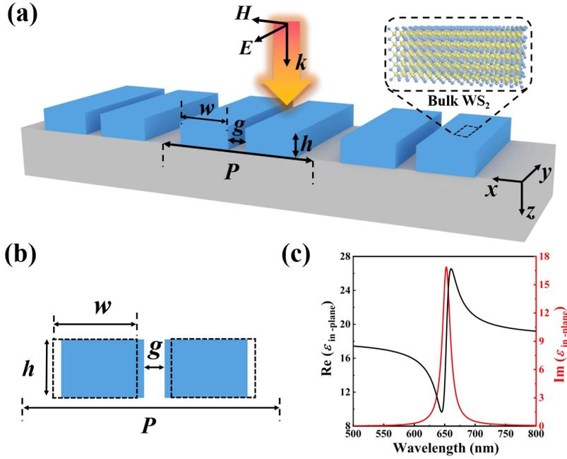
FIG. 1. (a) Schematic diagram of dimerized gratings composed of bulk WS<sub>2</sub>. (b) The  $xz$  cross-sectional of unit cell of the structure, with the dashed boxes corresponding to the case  $g = 145$  nm. (c) Real and imaginary parts of the in-plane dielectric function ( $\epsilon_{\text{in-plane}}$ ) of bulk WS<sub>2</sub>.
