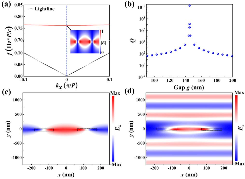
FIG. 2. (a) Band structure of the system associated with BIC. Inset: Normalized field distribution of BIC mode, where the black boxes indicate the structure. (b) The  $Q$ -factor of quasi-BIC as a function of gap  $g$ . The electric field ( $E_z$ ) of (c) BIC ( $g = 145$  nm) and (d) quasi-BIC ( $g = 127$  nm).
