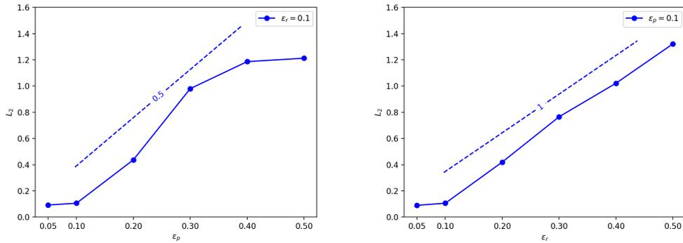
FIGURE 7. Error profiles when solving a 2D Poisson equation with one peak. Left: the prediction errors with respect to the  $\epsilon_p$  with  $\epsilon_r = 0.1$ . Right: the prediction errors with respect to the  $\epsilon_r$  with  $\epsilon_p = 0.1$ .
