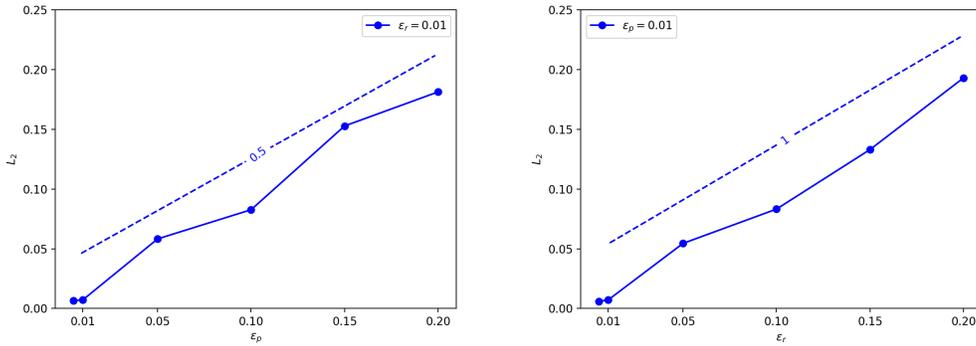
FIGURE 11. Errors profiles when solving Burgers' equation. Left: the prediction errors with respect to the  $\epsilon_p$  with  $\epsilon_r = 0.01$ . Right: the prediction errors with respect to the  $\epsilon_r$  with  $\epsilon_p = 0.01$ .
