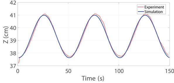
(c) Height  $z(t)$  of segment 2's tip in simulation and experiment.
