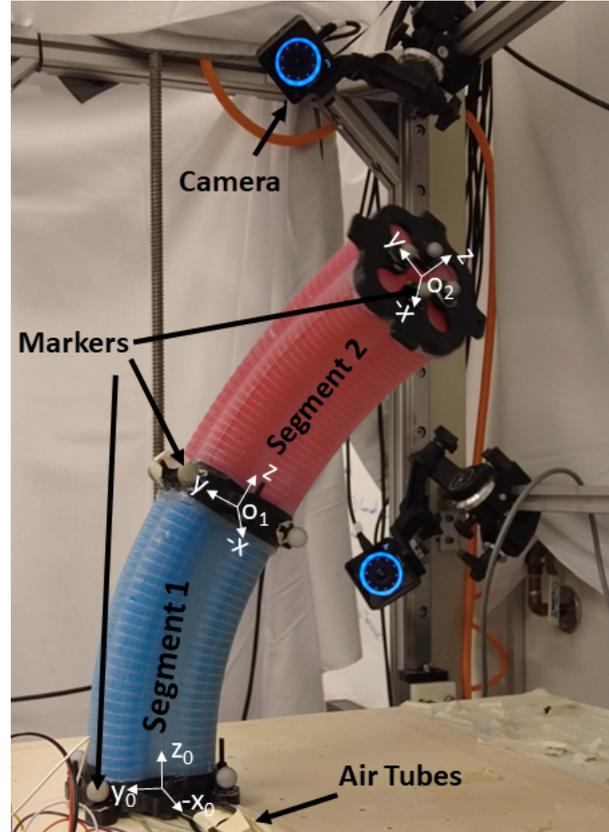
Fig. 1: The multi-segment silicone robotic arm used in this work. The silicone segments were fabricated using a method similar to the one in [1].
