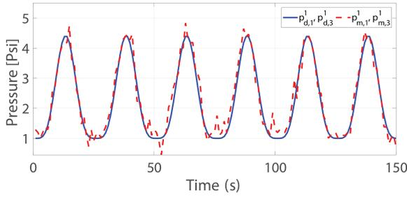
(e) Desired pressure  $p_{d,j}^1$  and measured pressure  $p_{m,j}^1$  for actuator  $j$  of segment 1 during the experiment.
