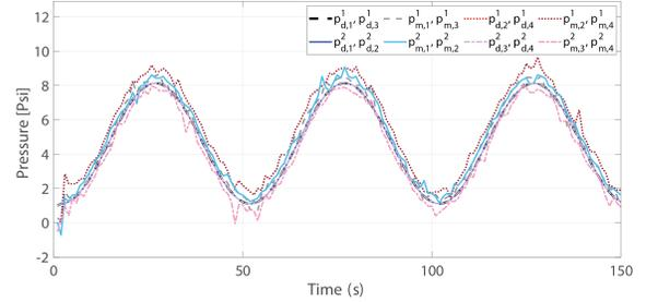
(d) Desired pressure  $p_{d,i,j}^i$  and measured pressure  $p_{m,i,j}^i$  for actuator  $j$  of segment  $i$  during the experiment.
