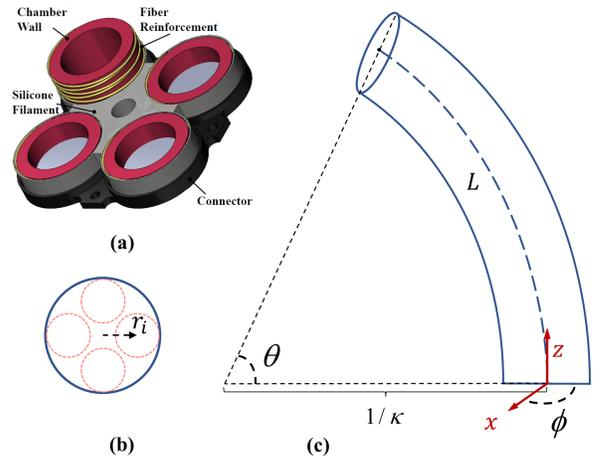
Fig. 2: (a) Design of a silicone segment. (b) Cross-section of a segment.  $r_i$  is the vector from the backbone to the center of the  $i$ -th FRA chamber in the local frame of the cross-section. The cross-section has area  $A$ , and the  $i$ -th FRA chamber has cap area  $A_i$ . (c) Kinematic representation of a constant-curvature segment with respect to a local frame fixed at the base of the segment.
