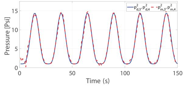
(f) Desired pressure  $p_{d,j}^2$  and measured pressure  $p_{m,j}^2$  for actuator  $j$  of segment 2 during the experiment.
