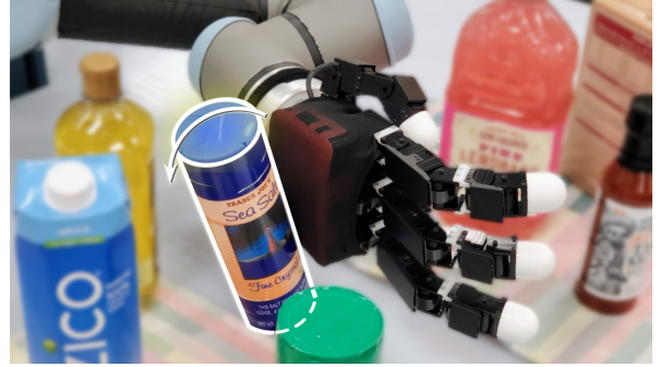
Fig. 1. When reaching through clutter, especially if the identity and mobility of objects are unknown, tactile sensors on surfaces such as the back of the hand can be used to prevent unsafe contact events, such as toppling an object.
