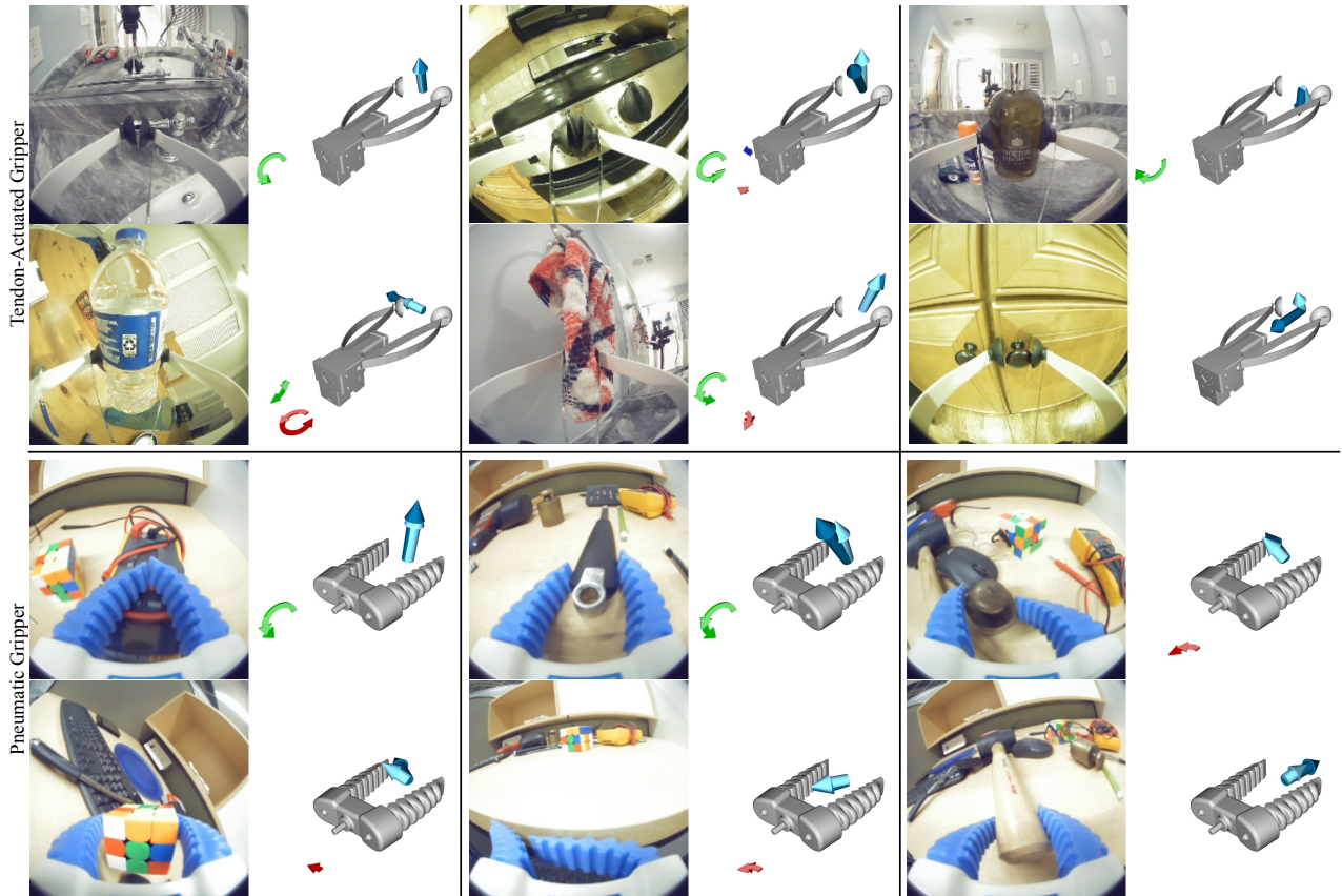
Fig. 3. Frames from the test set for both the tendon-actuated gripper and the pneumatic gripper are shown. Estimates from VFTS-Net are visualized as lightly shaded arrows, and ground truth measurements from the force/torque sensor are darkly shaded arrows. We collected data while the gripper was interacting with objects in a variety of environments, including a bathroom, kitchen, dining room, and office space. The bottom right figure for both gripper types shows a failure case. Both grippers estimate force in the Z-axis less accurately.
