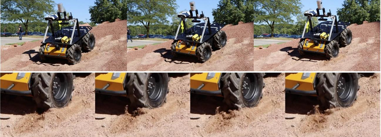
Fig. 5: A sequence of snapshots illustrating the substantial slip that is occurring during the experiment. If looking at the contact points of the right rear wheel with ground, one can observe that sands are rolling behind when the wheel is rotating.
