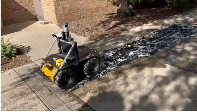
Fig. 2: The Husky robot is navigating on a highly slippery soap-covered tape ground (black areas).
