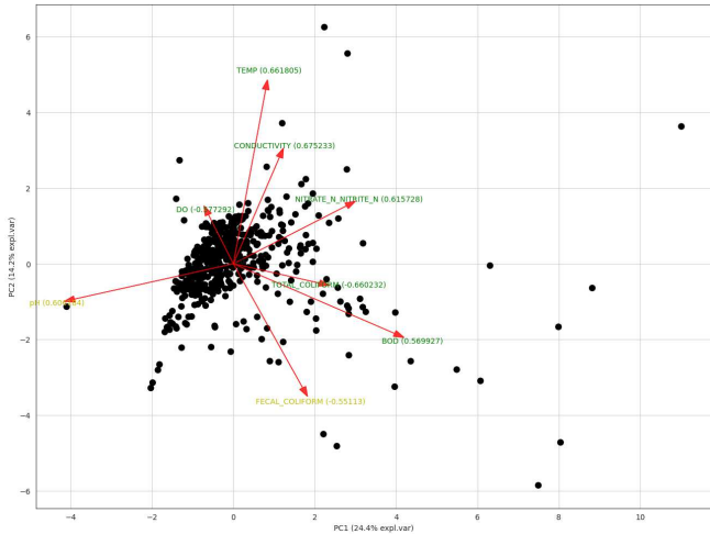
Fig. 3. Biplot of the PCA analysis on the first and second principal components. There is a strong correlation between Dissolved Oxygen, Fecal Coliforms, Total Coliforms and Nitrogen to BOD. pH and Fecal coliforms have no linear correlation toward each other
