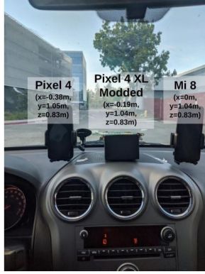
(a) Pixel 4 XL Modded smartphone used for data collection
