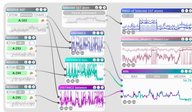
Fig. 8. A setup of the network during the first study. The rightmost sMolBoxes show from the top: the RMSD of the residues forming the tunnel bottleneck, throughput of the tunnel bottleneck loaded from an external CSV file, and comparison of the minimal distance of three ligands (IDs 293, 294, 295) to the residue in the active site (ID 103).
